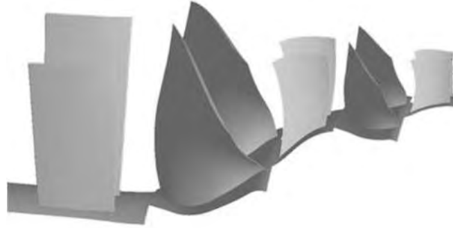
Figure 2 Two-stage highly loaded Fan model
