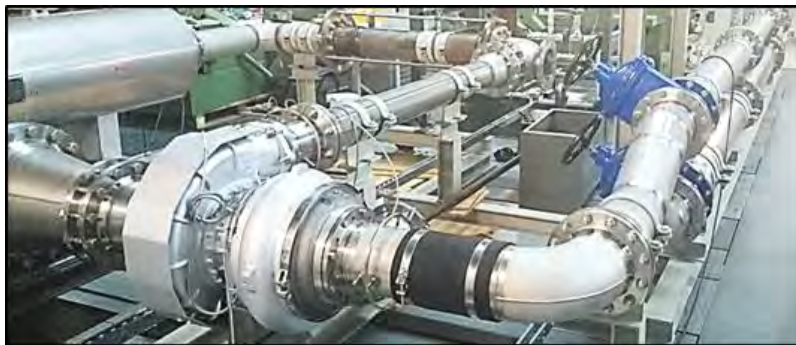
Figure 9: Turbocharger Test Rig at IKDG Institute, RWTH Aachen University
