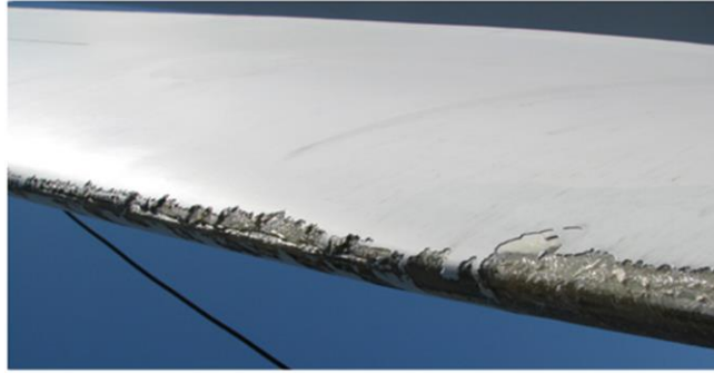
Figure 1 Erosion on the leading edge of a wind turbine blade (Source: Keegan et al. (2013)).
