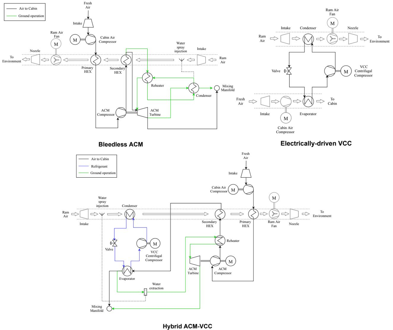
**Figure 1** Simplified process flow diagram of three novel environmental control system architectures.
