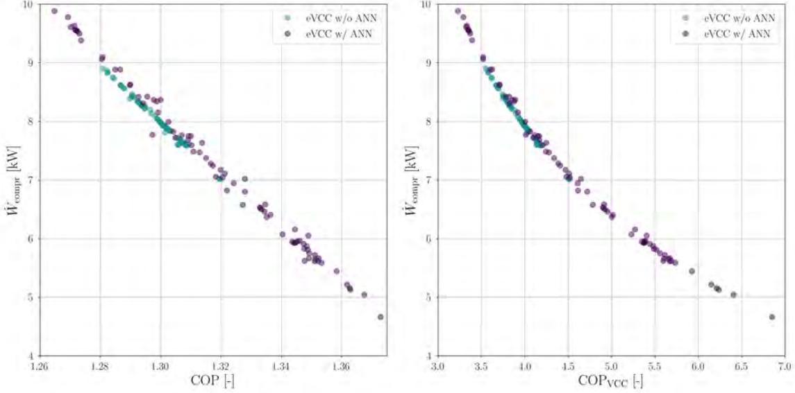
**Figure 9 Comparison between the trends of the refrigerant compressor mechanical power vs. the COP of the ECS (left), and of the VCC system (right), computed with and without the use of the data-driven compressor model.**
