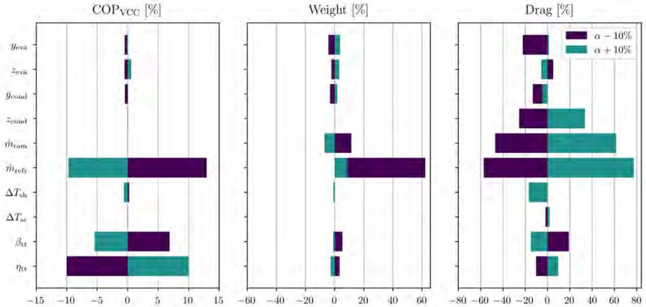
**Figure 10 Sensitivity of the objective functions with respect to a  $\pm 10\%$  perturbation in the vector of design variables. The analysis is repeated for five optimal design points selected over the Pareto front identified with the modified optimization framework, and the results are averaged.**
