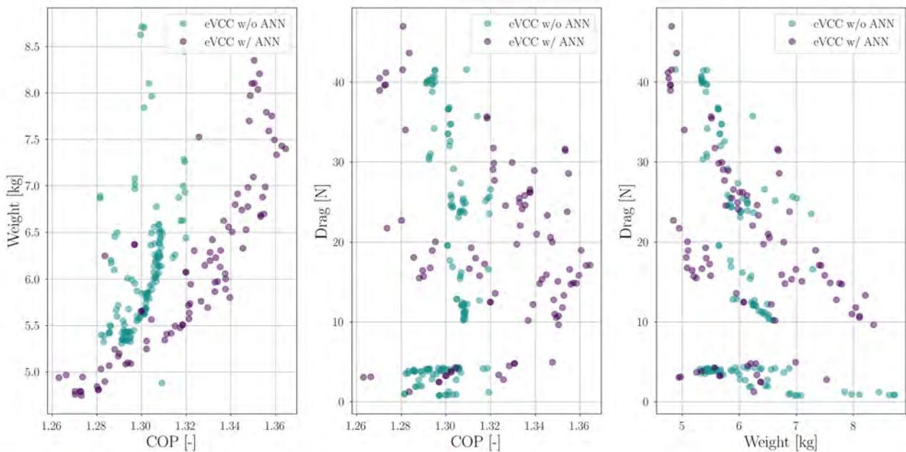
**Figure 8** Comparison between the trends established among the objective functions, computed with and without the use of the data-driven compressor model, coupled to the integrated design optimization framework.
