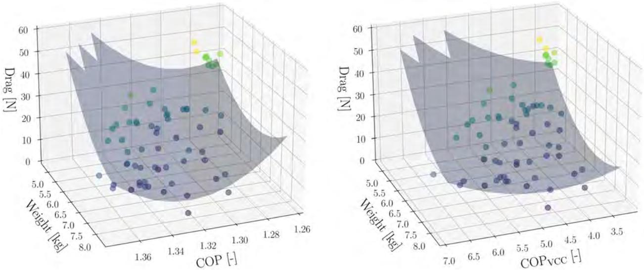
**Figure 7** Pareto front computed with the modified optimization framework coupled to the data-driven compressor model, considering the COP of the entire ECS (left), and the COP of the VCC system (right).
