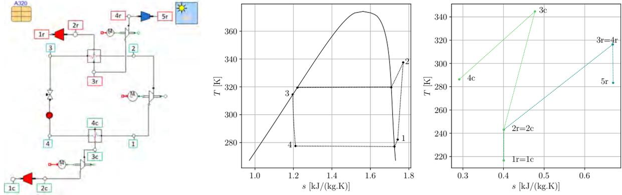
**Figure 2** Modelica model of the electrically-driven VCC system.  $T - s$  chart reproducing the thermodynamic processes occurring in the refrigeration loop (left chart), and in the ram and cabin air ducts (right chart).
