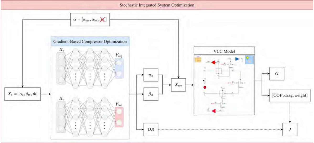
**Figure 6** Flowchart of the modified ECS optimization framework. The data-driven model is used to decouple the optimization of the high-speed centrifugal compressor, highlighted in blue, from the optimization of the VCC system, highlighted in red.
