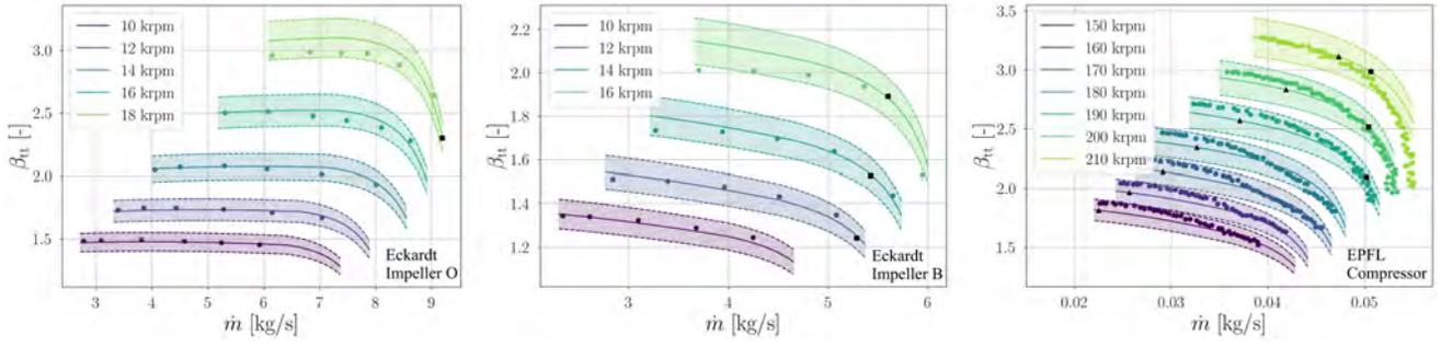
**Figure 3 Validation of the in-house compressor model with experimental data. Solid lines represent compressor model predictions; dashed lines bound colored  $\pm 5\%$  uncertainty bands; dots correspond to experimental data of Eckardt impellers O and B Eckardt (1977); Japikse (1987), and EPFL compressor Schiffmann and Favrat (2010). The estimated choking and rotating stall operating points are marked by  $\blacksquare$  and  $\blacktriangle$ , respectively.**
