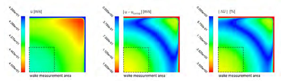
Figure 5 Schematic procedure for determining the percentage velocity variation on the contraction outlet plane
