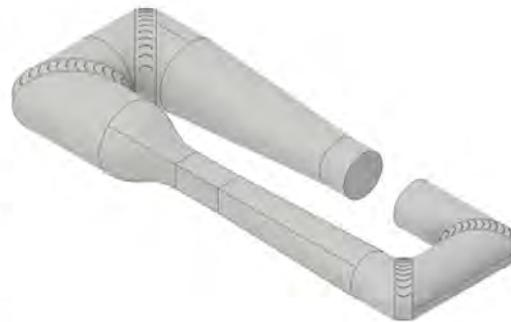
**Figure 2 Wind tunnel Göttingen-Type closed test section configuration**
