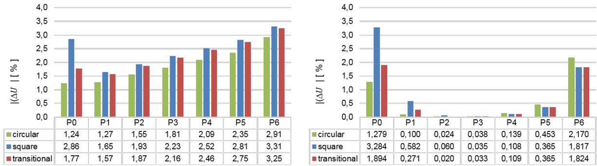
Figure 7 Percentage velocity variation of the entire (left) and partial evaluation planes (right)
