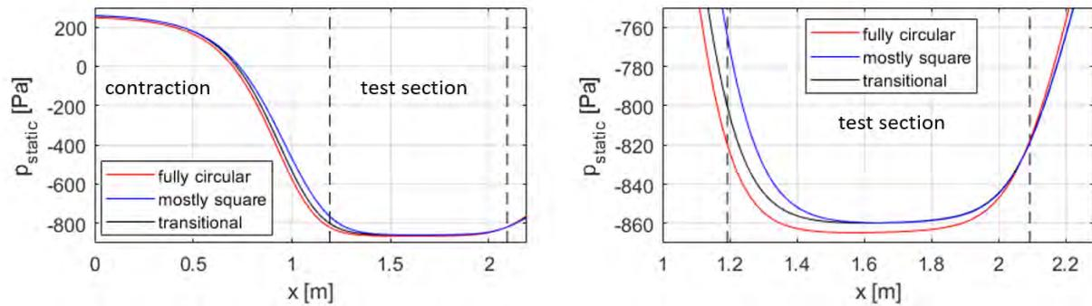
Figure 8 Static pressure distribution on the central axes
