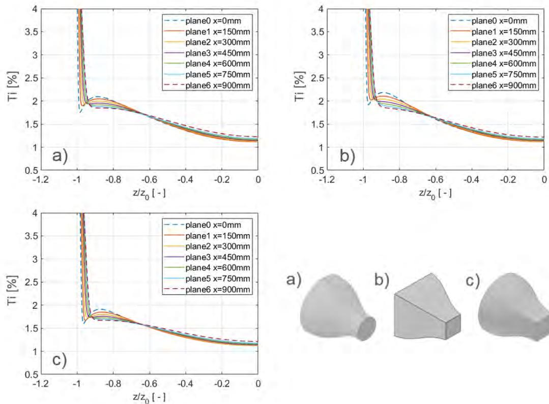
**Figure 9** Turbulence intensity on symmetry planes for the a) fully circular b) mostly square and c) transitional wind tunnel setup
