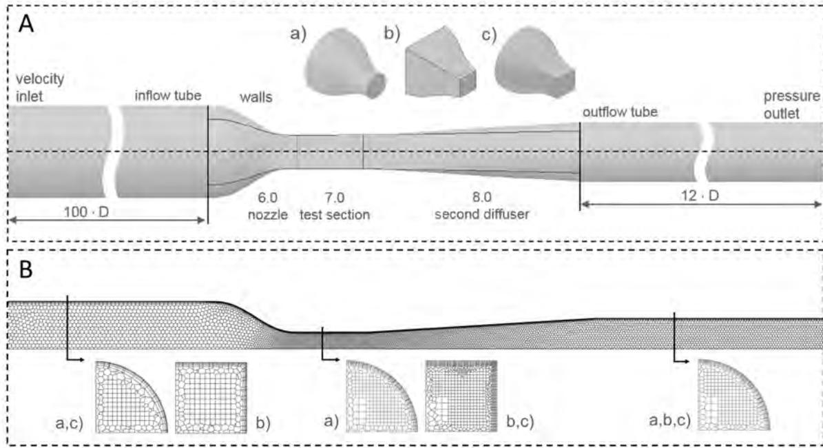
**Figure 3 A) Computational domain for the simplified wind tunnel setup with a) circular shaped b) square shaped c) transitional nozzle geometry and B) illustration of the applied unstructured mesh**
