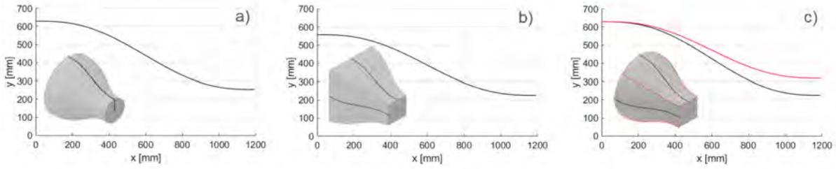
Figure 4 Nozzle geometries generated by a) rotation b) extrusion c) loft function
