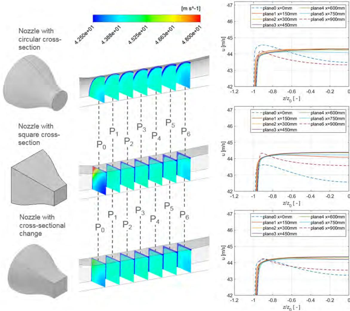
Figure 6 Velocity distribution on the evaluation and symmetry planes
