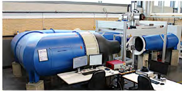
**Figure 1 Wind tunnel Göttingen-Type open test section configuration**
