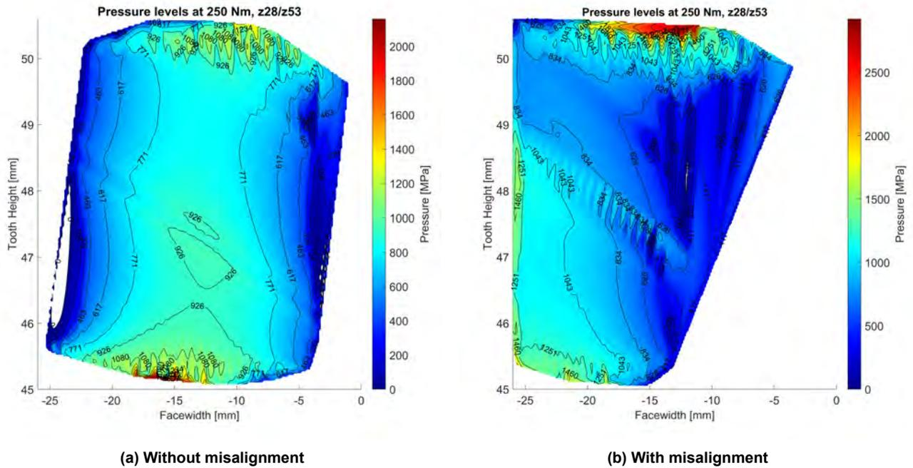
Figure 8 Contact pressures along the active flank, first set of profile modifications
