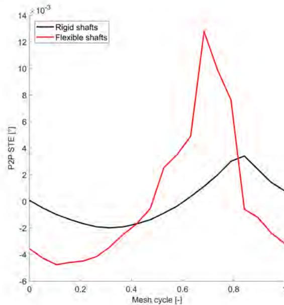
Figure 9 STE comparison with and without misalignment, second set of profile modifications.
