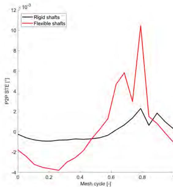
**Figure 7 STE comparison with and without misalignment, first set of profile modifications.**
