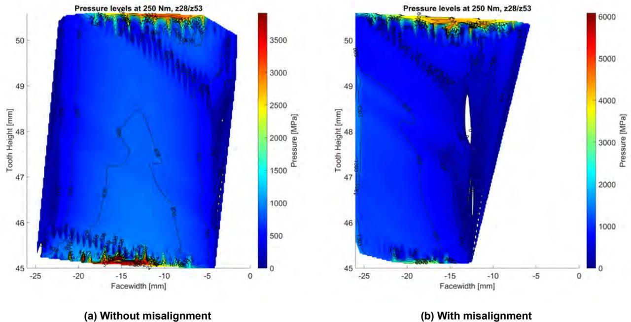
**Figure 6 Contact pressures along the active flank, without profile modifications**
