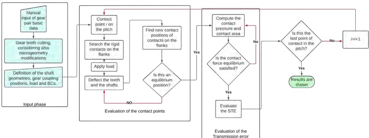
Figure 3 Flowchart of the numerical procedure
