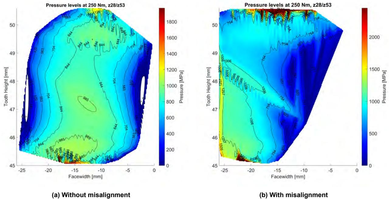
**Figure 10 Contact pressures along the active flank, second set of profile modifications**
