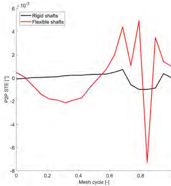
**Figure 5 STE comparison with and without misalignment, without profile modifications.**
