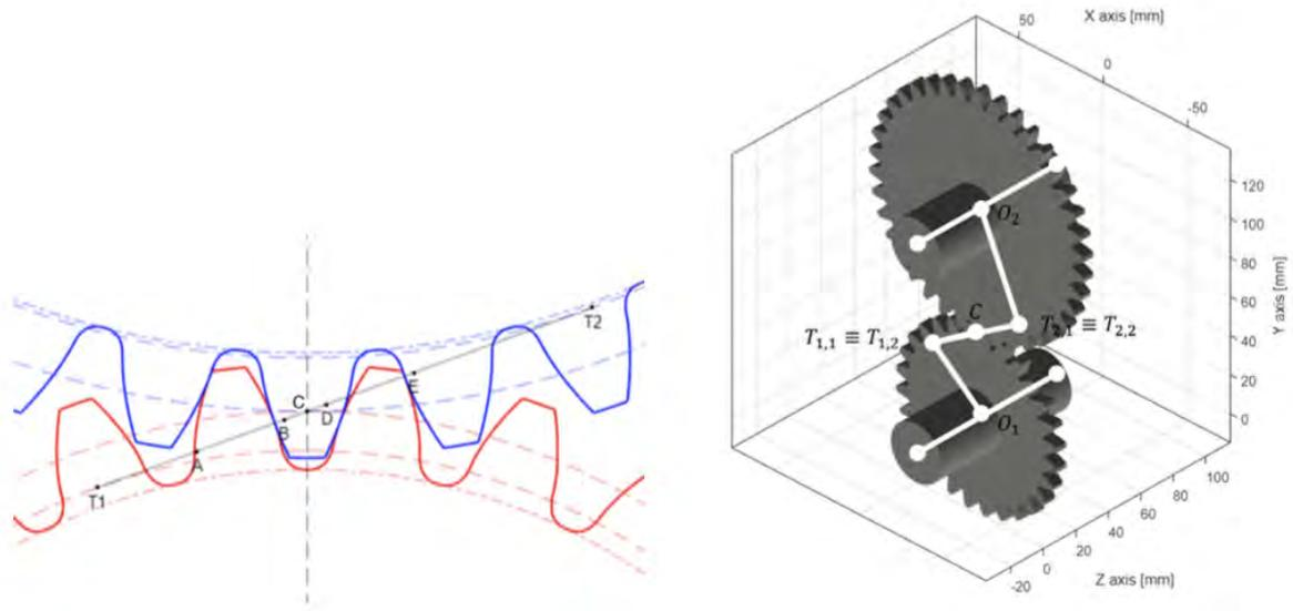
Figure 2 Scheme for links between shafts that depicts the gear set
