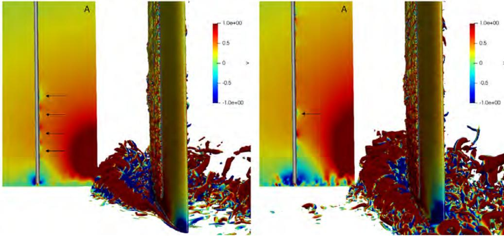
Figure 7 Mean spanwise velocity contour at plane A and interaction with the TLV - (left): moving end-wall; (right): stationary end-wall.
