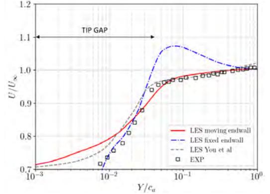
**Figure 5** Profiles of the mean streamwise velocity at  $X/c_a = 0$  and  $Z/c_a = 0$ .
