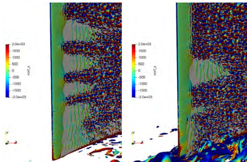
**Figure 6** Iso-surfaces of Q-criterion ( $1.0 \times 10^6 \text{ s}^{-2}$ ) on the blade PS at the tip close to the LE: boundary layer development - (left): moving end-wall; (right): stationary end-wall.
