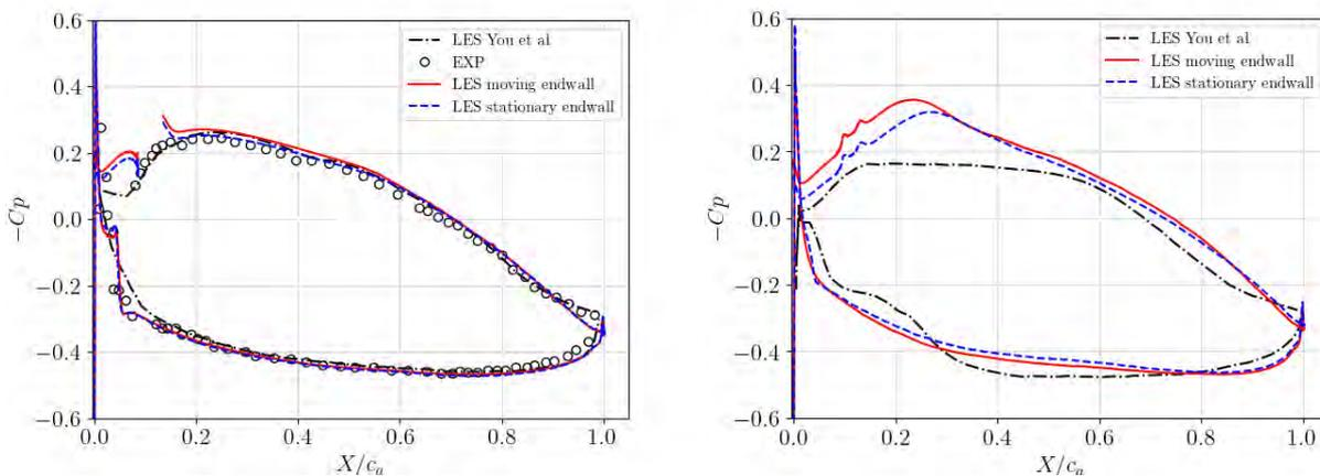
Figure 8 Pressure coefficient evaluated at midspan (left) and at  $10\%C_a$  away from the blade tip (right).
