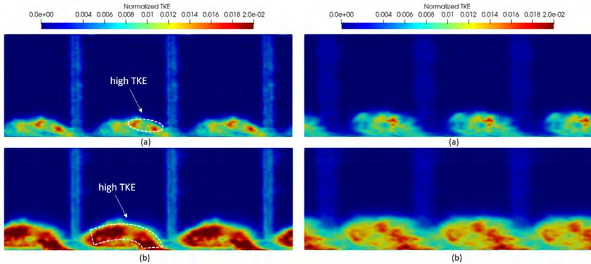
**Figure 11 Normalized turbulent kinetic energy at  $X/c_a = 1.37$  (left) and  $X/c_a = 2.06$  (right) - (a): moving endwall (b): stationary endwall.**
