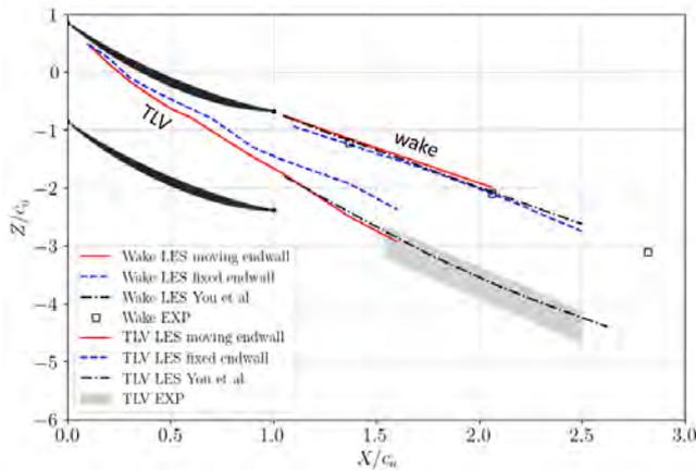
**Figure 13** Tip leakage vortex and wake trajectories on the  $(X,Z)$  plane.
