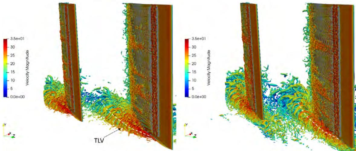
Figure 4 Iso-surfaces of  $Q$ -criterion ( $1.0 \times 10^6 \text{ s}^{-2}$ ) coloured by the velocity magnitude - (left): moving end-wall; (right): fixed end-wall.
