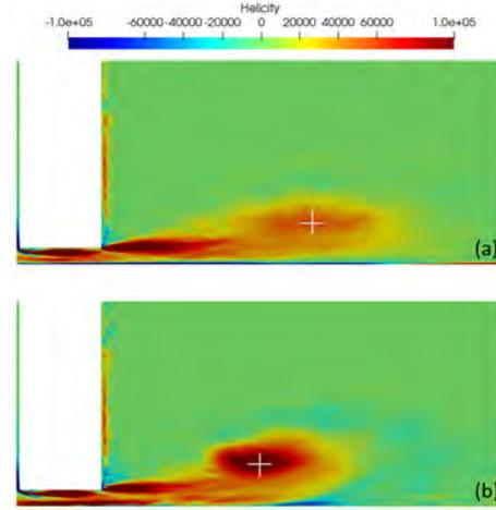
**Figure 14** Mean helicity contours in the TLV region at  $X/c_a = 0.4$  - (a): moving end-wall; (b): fixed end-wall.
