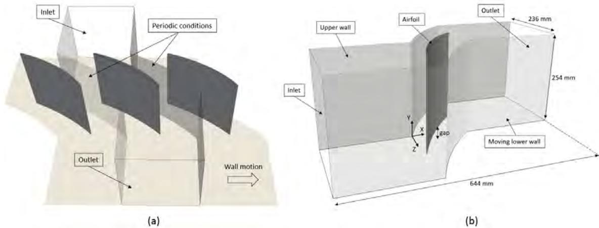
Figure 2 Numerical domain - (a): compressor cascade; (b): single passage and reference system.
