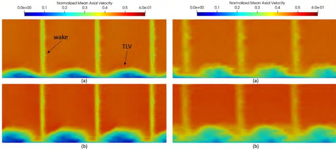
Figure 10 Normalized mean axial velocity at  $X/c_a = 1.37$  (left) and  $X/c_a = 2.06$  (right) - (a): moving end-wall (b): stationary end-wall.
