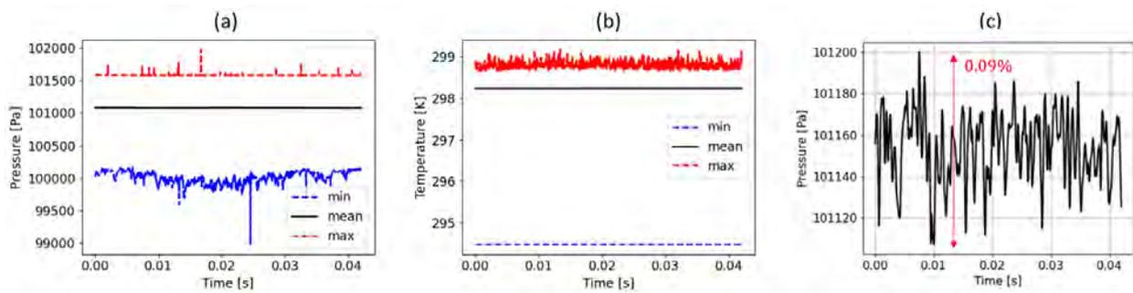
Figure 3 Convergence - (a)/(b) : time evolution of maximum, mean and minimum values for (a) global pressure and (b) temperature; (c) : pressure signal on the blade SS at midspan.
