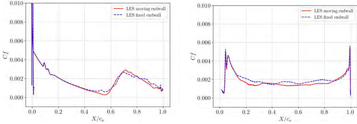
Figure 9 Friction coefficient evaluated at midspan at the blade SS (left) and PS (right).
