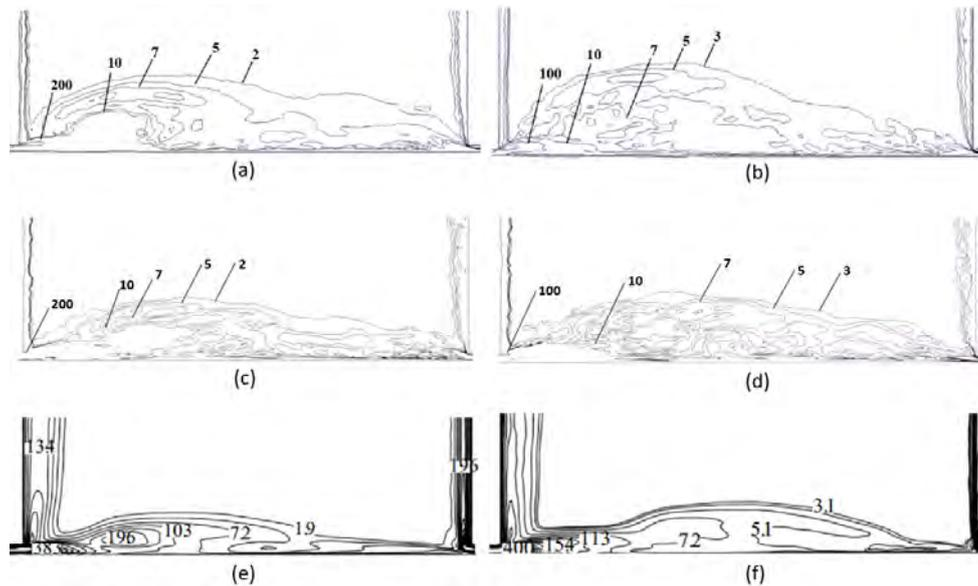
**Figure 12 Iso-lines of normalized mean vorticity magnitude. Comparison between LES by Koch (above), present LES (middle) and LES by You et al (below) - (a)/(c)/(e):  $X/c_a = 0.5$  and (b)/(d)/(f):  $X/c_a = 0.7$ .**
