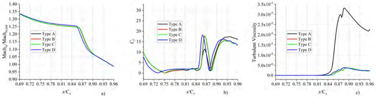
**Figure 9 Distributions of flow variables on the blade for  $k^+ = 8$ : a) isentropic Mach number; b) skin friction coefficient; c) turbulent viscosity.**
