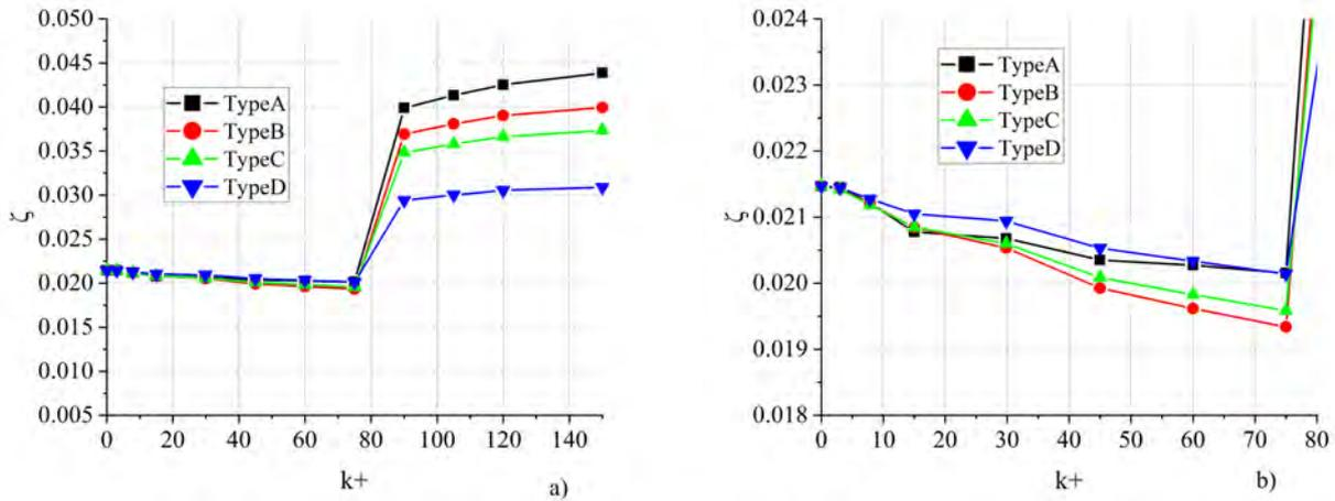
Figure 7 Variations of KELC versus  $k^+$ : a) global; b) locally enlarged
