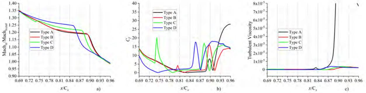
**Figure 11 Distributions of flow variables on the blade for  $k^+ = 75$ : a) isentropic Mach number; b) skin friction coefficient; c) turbulent viscosity.**
