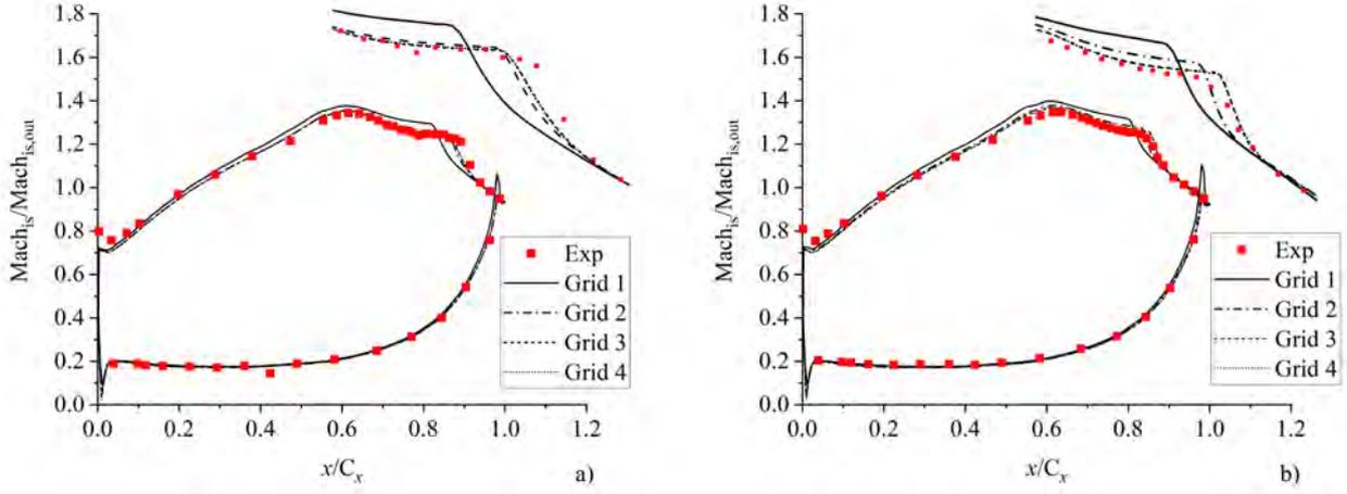
**Figure 4 Isentropic Mach number distributions on the blade: a)  $Re = 1.4 \times 10^5$ ; b)  $Re = 2.5 \times 10^5$**
