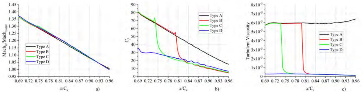
**Figure 12 Distributions of flow variables on the blade for  $k^+ = 120$ : a) isentropic Mach number; b) skin friction coefficient; c) turbulent viscosity.**
