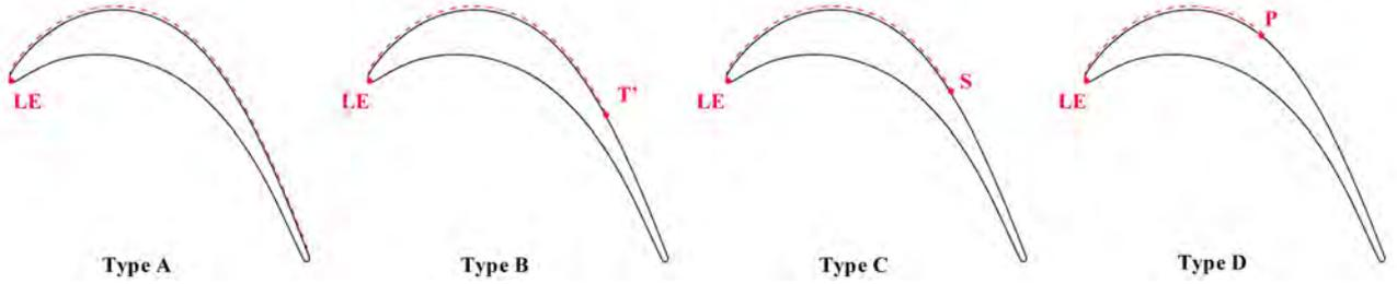
**Figure 5 Roughness allocations on the suction side**
