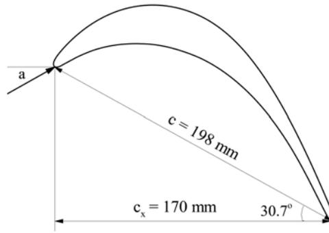
**Figure 1 Profile of T106C cascade**
