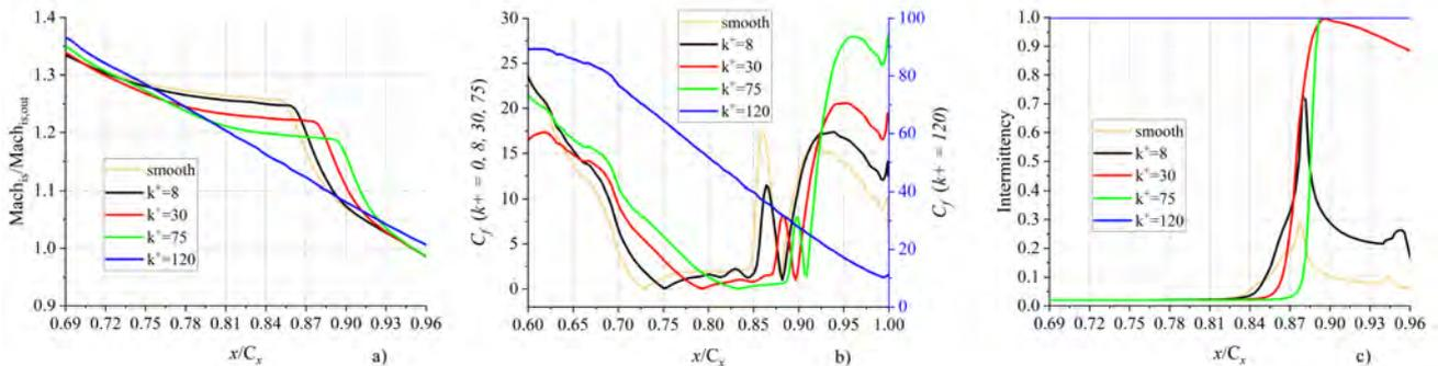
Figure 8 Distribution of flow variables on the blade: a) isentropic Mach number; b) skin friction coefficient; c) intermittency
