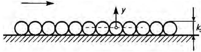
**Figure 6 Illustration of equivalent sand-grain roughness**
