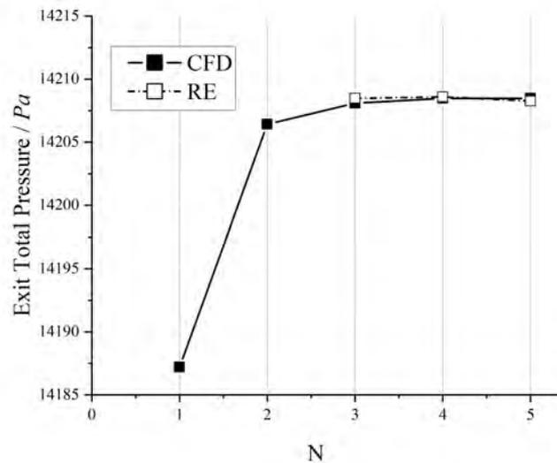
**Figure 3 Grid-independent solutions of outlet total pressure**
