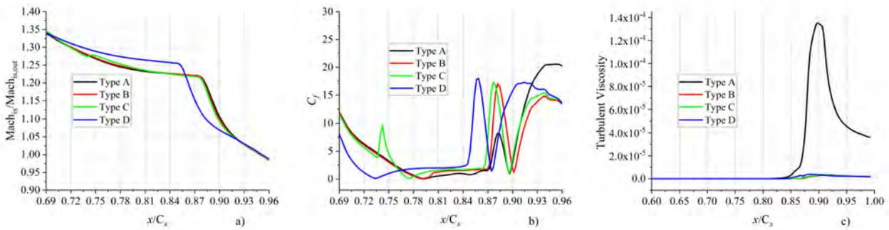
**Figure 10 Distributions of flow variables on the blade for  $k^+ = 30$ : a) isentropic Mach number; b) skin friction coefficient; c) turbulent viscosity.**
