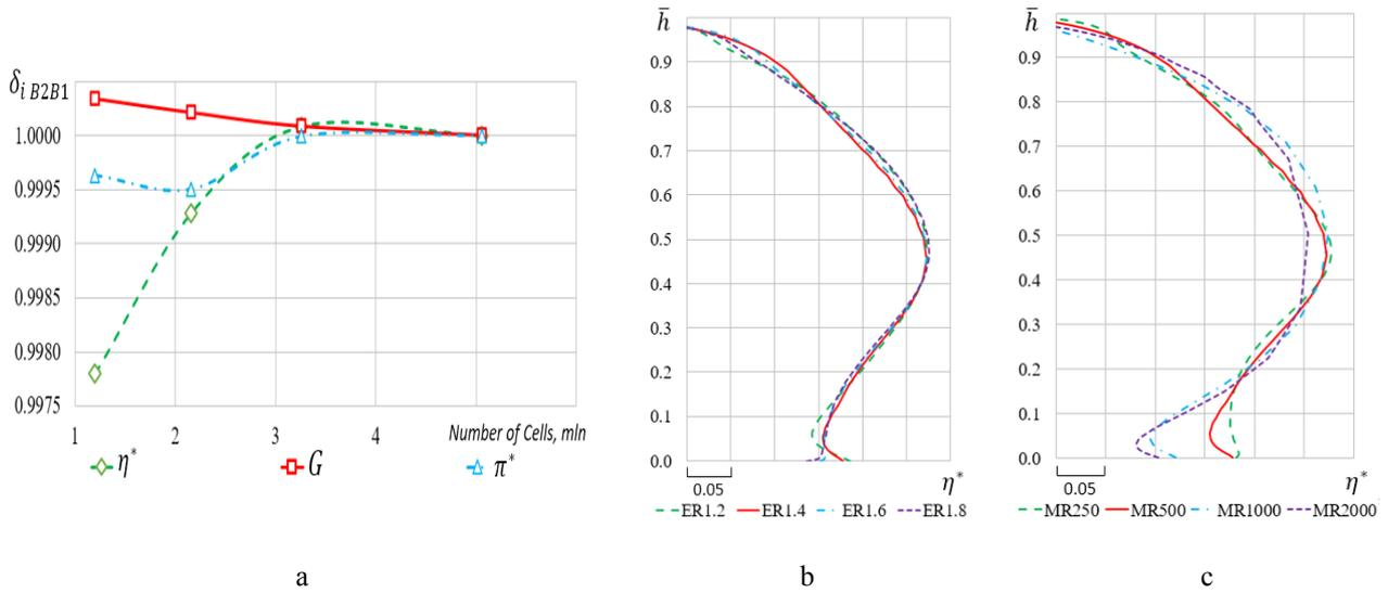
**Figure 4 Influence of the selected parameters on the working process modelling of the investigated turbine: a - B2B; b - ER; c - MR**
