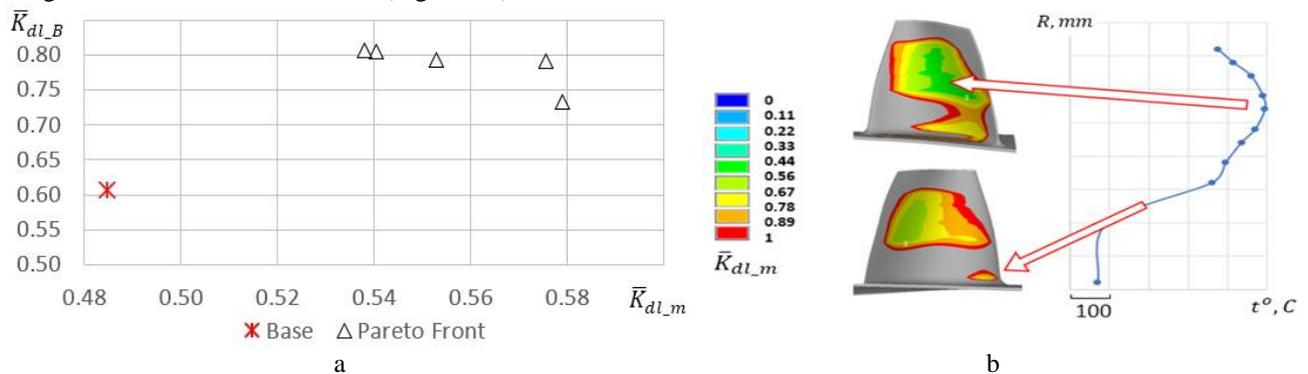
**Figure 8 Task of RW finishing of CT step 1: a - Pareto front, b - distribution of local strength reserve depending on the RW temperature**
