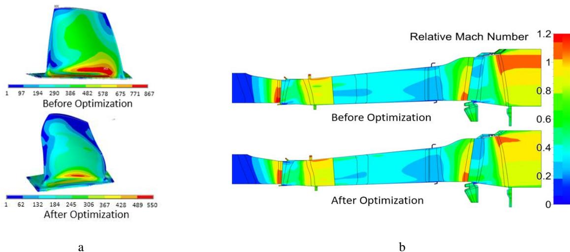
**FIGURE 11 COMPARISON OF CT PARAMETERS BEFORE AND AFTER OPTIMIZATION: A - AVERAGE MISES STRESSES IN RW, B - FIELDS OF RELATIVE MACH NUMBER**
