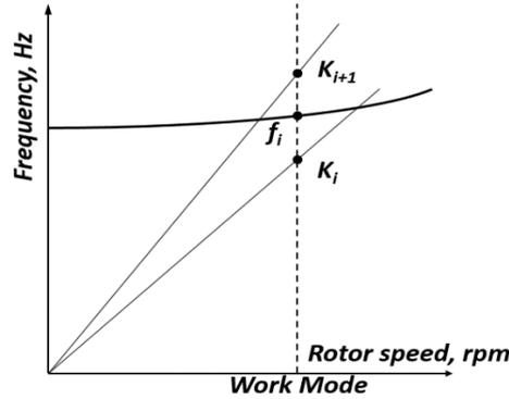
**Figure 6 Determination of a parameter  $\Delta f_i$  at Campbell diagram**
