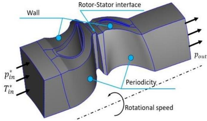
**Figure 3 Numerical model of a compressor turbine working process with boundary condition**
