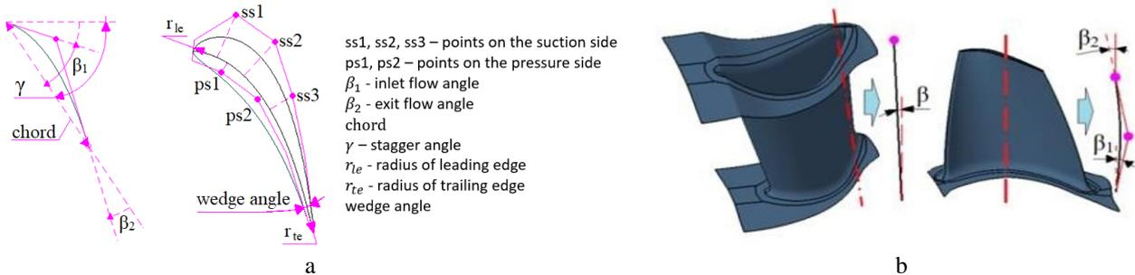
**Figure 7 Scheme of turbine blade parameterization**
