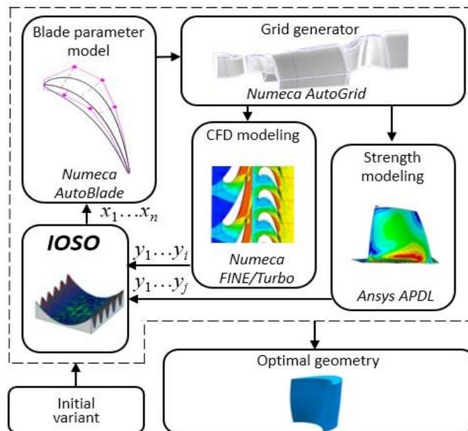
**Figure 2 Process chain used in the research.**
