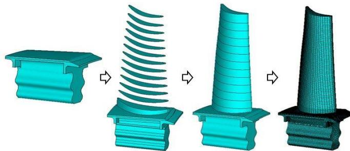
**Figure 5 A process for creating a strength model of CT working blade**
