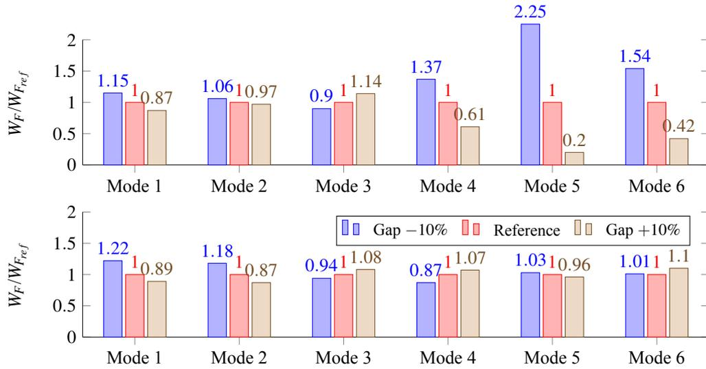
Figure 4 Relative aerodynamic work (top: OP1, bottom: OP3)
