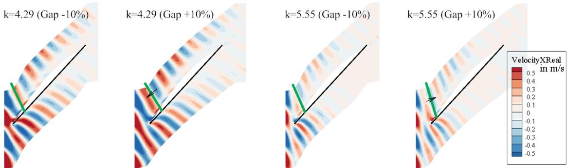
Figure 8 Real part of axial velocity at the midspan
