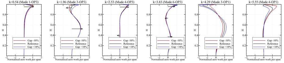
Figure 7 Radial distribution of chordwise-integrated aerodynamic work
