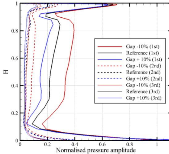
**Figure 3 Amplitude of unsteady pressure in the gust boundary conditions at the rotor inlet**
