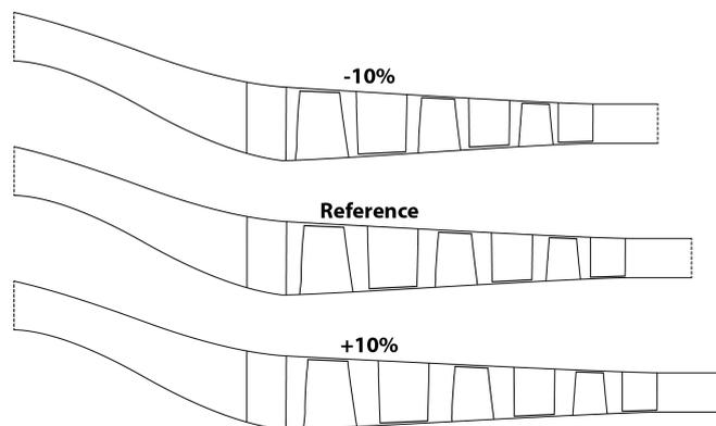
Figure 1 Different axial gaps in the meridional view (Eggers et al., 2020)
