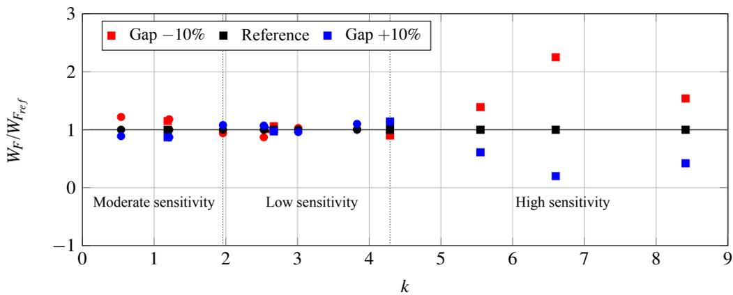
Figure 5 Relative aerodynamic work versus reduced frequency
