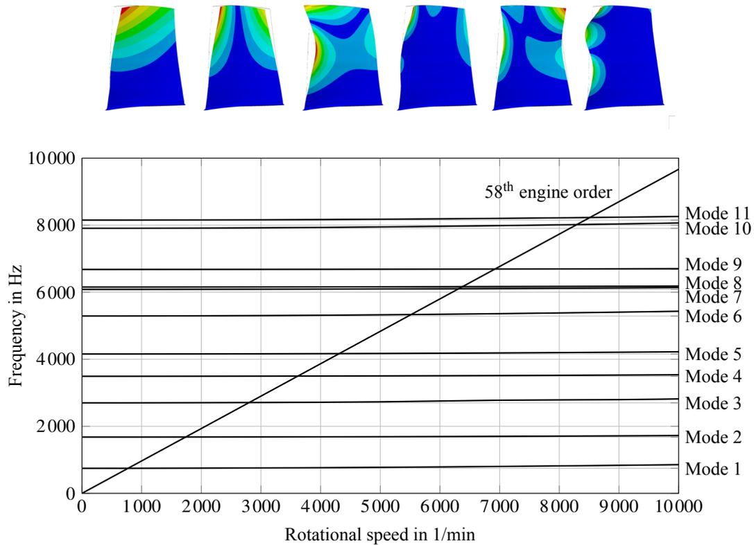
**Figure 2 Mode shapes of the rotor blade for Mode 1 to Mode 6 (blue - no deformation, red - maximum deformation) and Campbell diagram**
