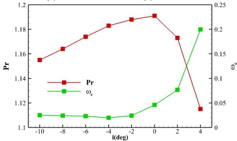
**Figure 2 Incidence Characteristic of Tandem Cascade**
