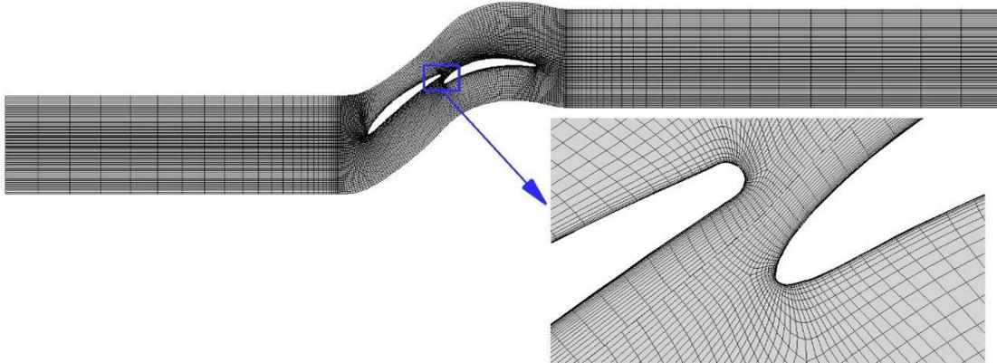
**Figure 1 Schematic Diagram of Single-channel Grid**
