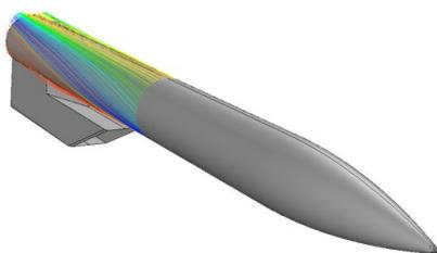
Fig. 11 Flow line of wall area ( $\alpha = 6^\circ$ )
