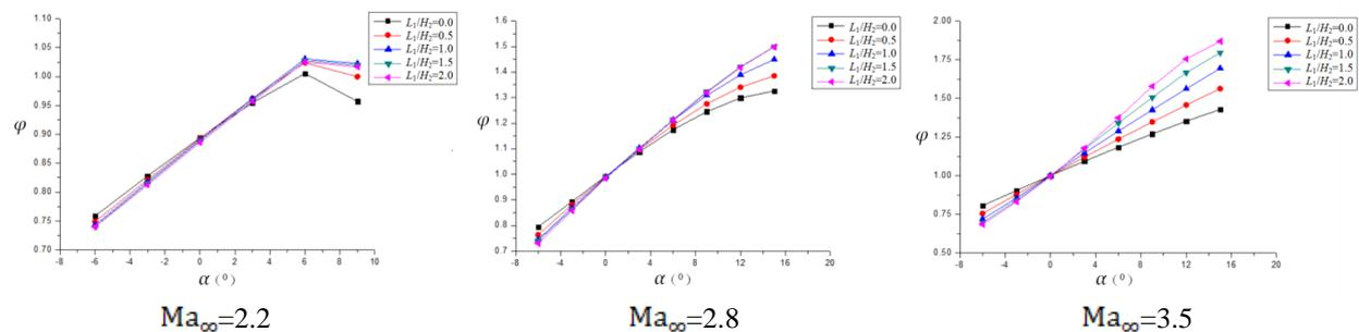
Fig. 9 Variation of flow coefficient with attack angle
