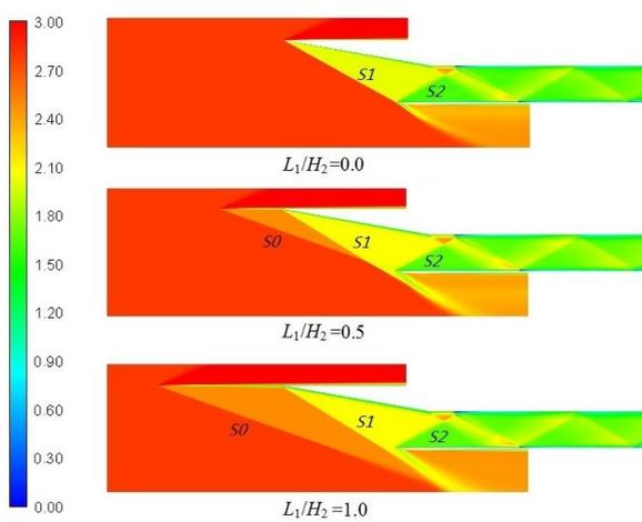
Fig. 6 Mach number distribution of different shield plate length ( $\alpha = 6^\circ$ )
