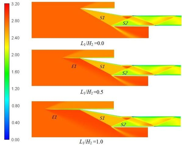
Fig. 7 Mach number distribution of different shield plate length ( $\alpha = -3^\circ$ )
