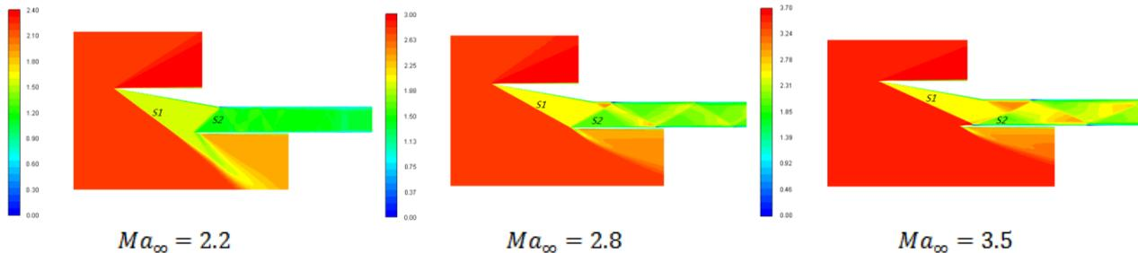
Fig. 5 Mach number distribution at 6 degrees of attack angle
