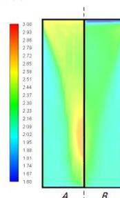
Fig. 12 comparison of Mach number of inlet section ( $\alpha = 6^\circ$ )
