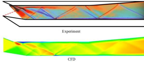
Fig.4 Comparison of Mach number distribution between experimental schlieren and numerical calculation
