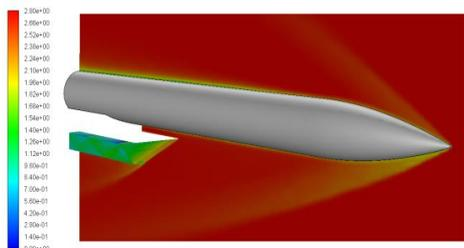
Fig. 10 Mach number distribution in symmetry plane ( $\alpha = 6^\circ$ )
