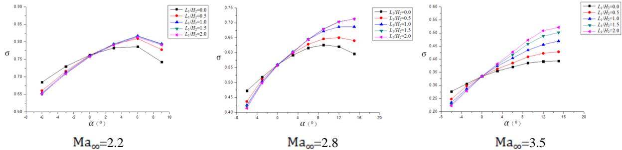
Fig. 8 Variation of total pressure recovery with attack angle
