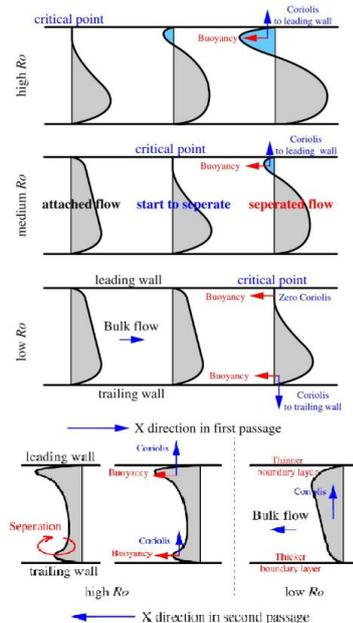
**Figure 4 flow profile of U-shaped square smooth passage under different rotation number ([Deng, et al. 2013](#))**
