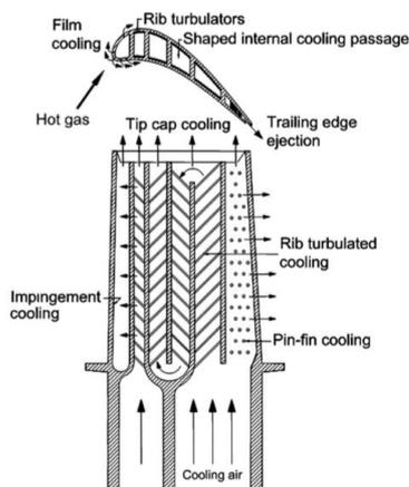
Figure 1 structure of serpentine passages in rotor blade (Je-Chin, 2004)
