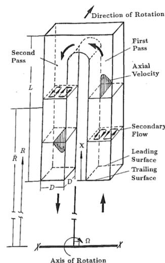
**Figure 3 Conceptual view of effect of Coriolis force and buoyance on flow profile ([Je-Chin, et al. 1993](#))**
