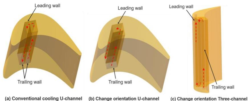
**Figure 6 Concept geometry of internal cooling channel in a rotor blade**
