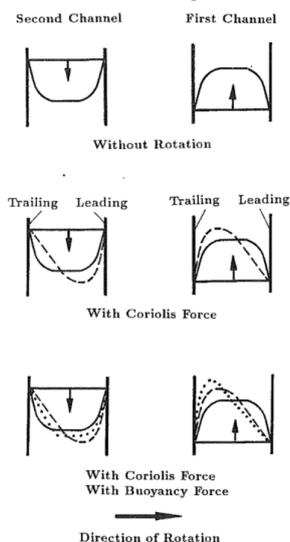
**Figure 2 Conceptual view of secondary flow and axial velocity distribution in a U-shaped rectangular smooth passage without heating under rotating condition ([Je-Chin, et al. 1993](#))**
