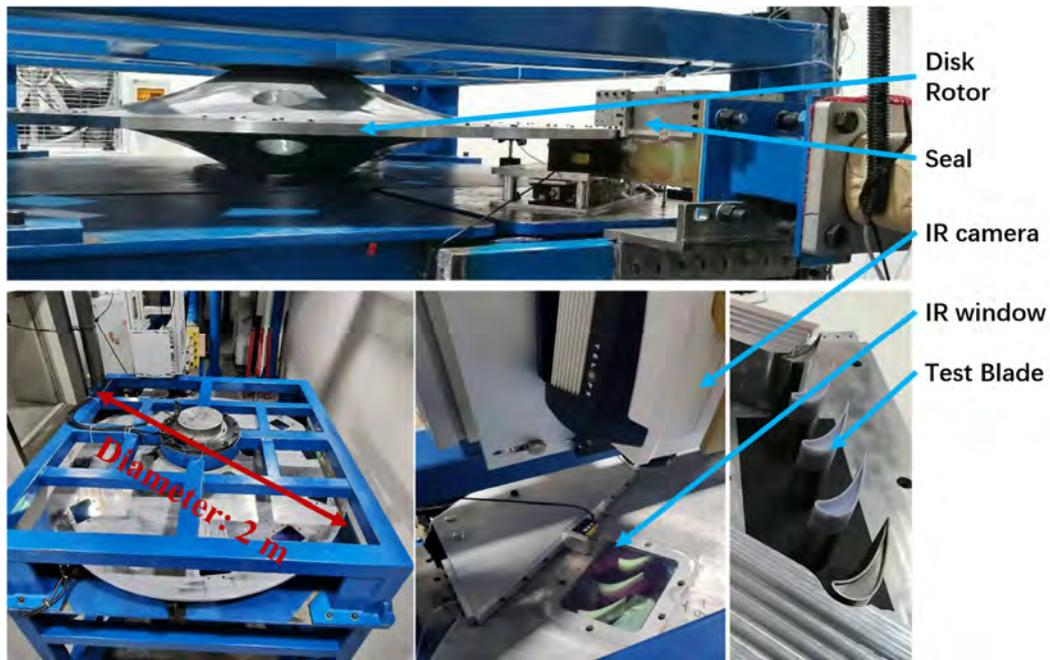
Figure 3 Details of disk rotor and test section
