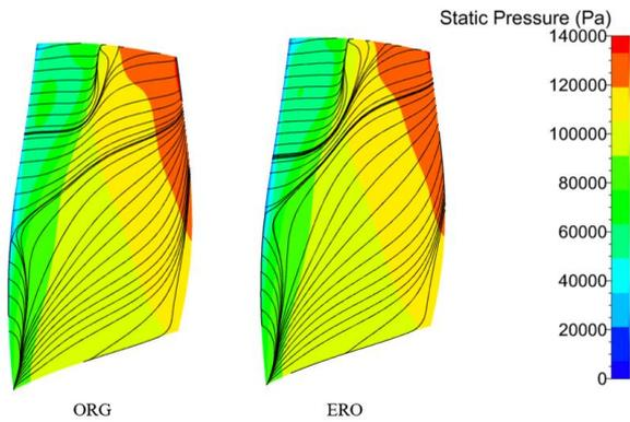
**Figure 12 Limit streamline of the suction side near stall point**
