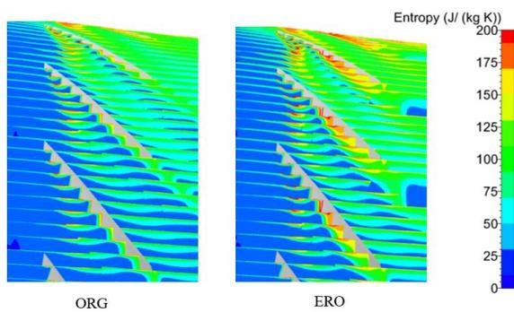
**Figure 18 Entropy distribution contour of blade tip near stall point**
