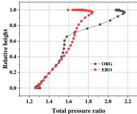
**Figure 10 Radial distribution of total pressure ratio near stall point**
