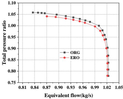
**Figure 6 Comparison of flow-total pressure ratio of two blades**
