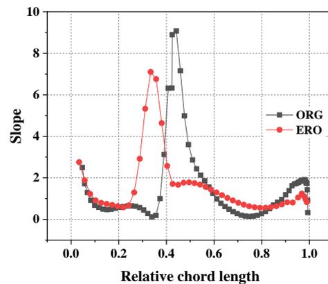
**Figure 15 Slope of static pressure coefficient**
