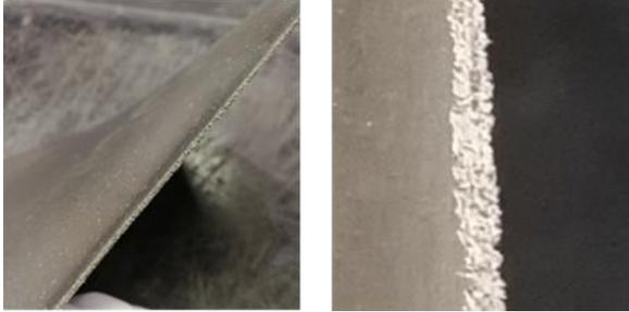
Figure 2 Overall shape and partial enlargement of the eroded blade leading edge
