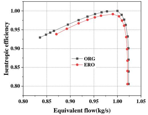
**Figure 7 Comparison of flow-isentropic efficiency of two blades**
