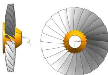
**Figure 1 Fan rotor component of a high bypass ratio engine**
