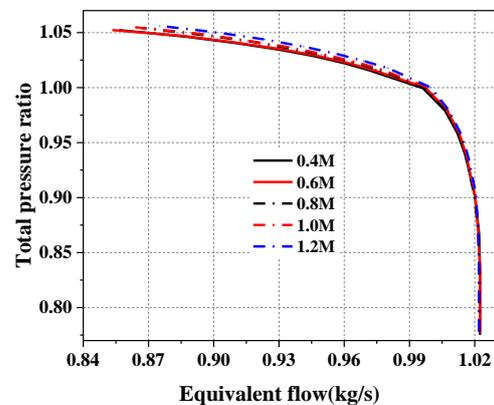
Figure 5 Grid independence check of flow-total pressure ratio
