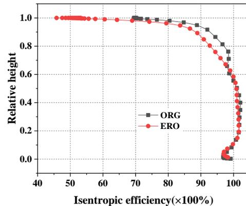
**Figure 11 Radial distribution of isentropic efficiency near stall point**
