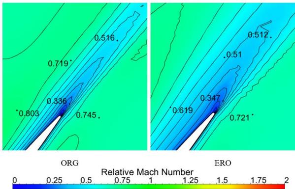
**Figure 16 Wake distribution contour of 95% relative height near stall point**
