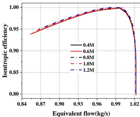
Figure 4 Grid independence check of flow - isentropic efficiency
