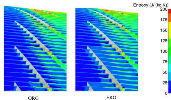
**Figure 19 Entropy distribution contour of blade tip at design point**
