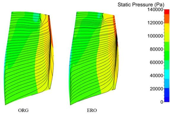
**Figure 13 Limit streamline of the suction side at design point**
