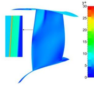
Figure 3  $y^+$  value of rotor wall
