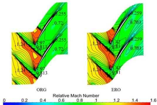
**Figure 8 Relative Mach number contour of 95% relative height near stall point**
