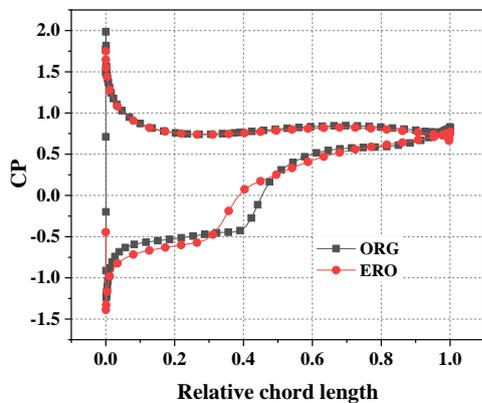
**Figure 14 Surface static pressure coefficient distribution of 95% relative height near stall point**
