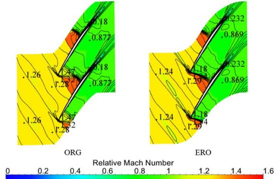
**Figure 9 Relative Mach number contour of 95% relative height at design point**
