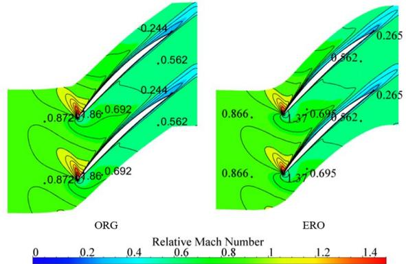
**Figure 17 Relative Mach number contour of 50% relative height near stall point**
