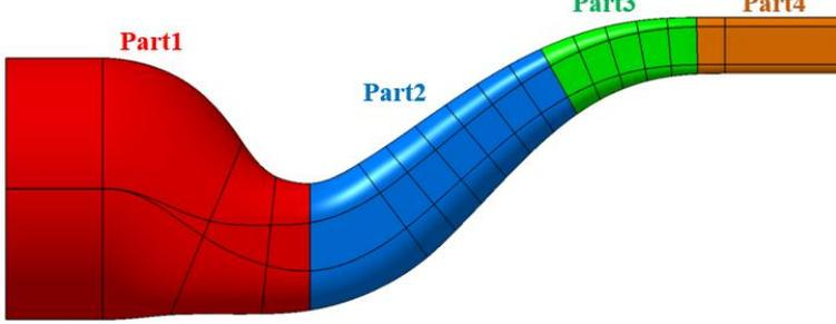
Figure 10 Schematic Diagram of 4 Parts in Serpentine Nozzle
