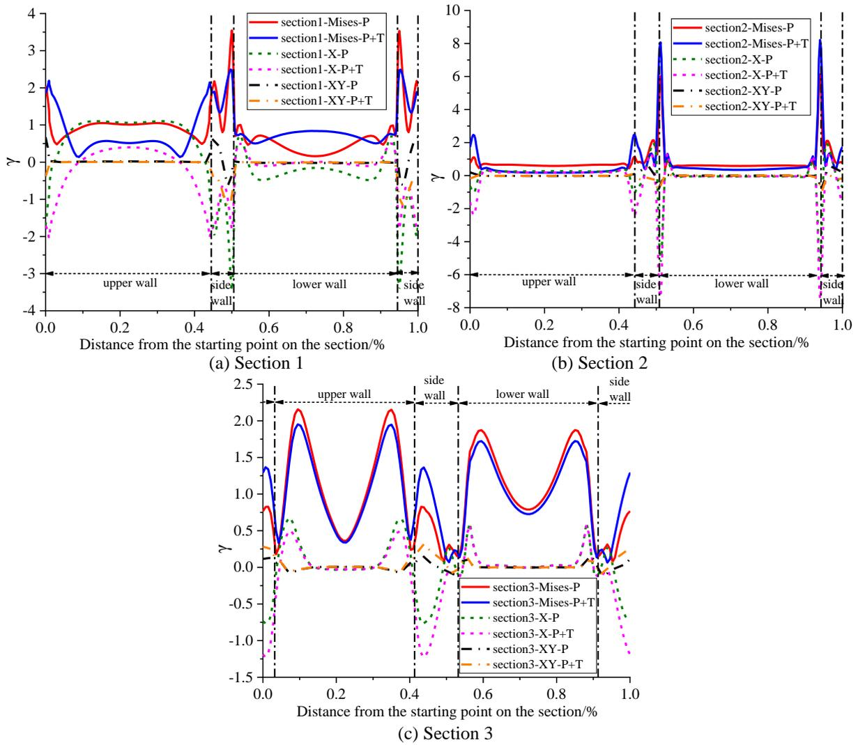
**Figure 8 Shear Lag Coefficient Curve under Different Load Conditions on Sections 1, 2, and 3**
