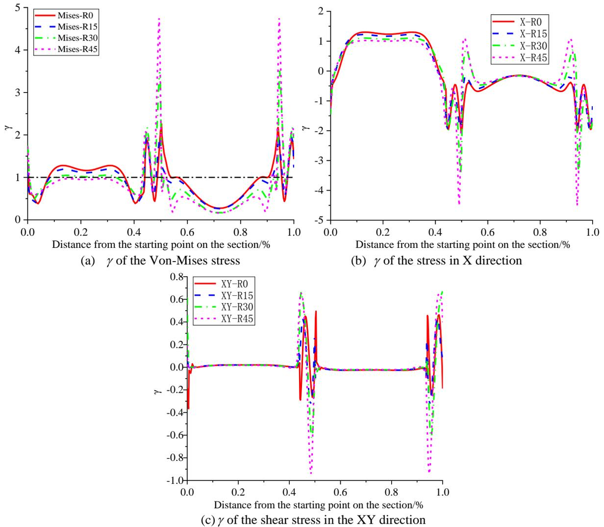
**Figure 7 Shear Lag Coefficient Curves of Models with Different Fillet Sizes on Section 1**
