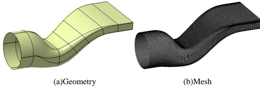
Figure1 Geometry and Mesh of the Serpentine Nozzle
