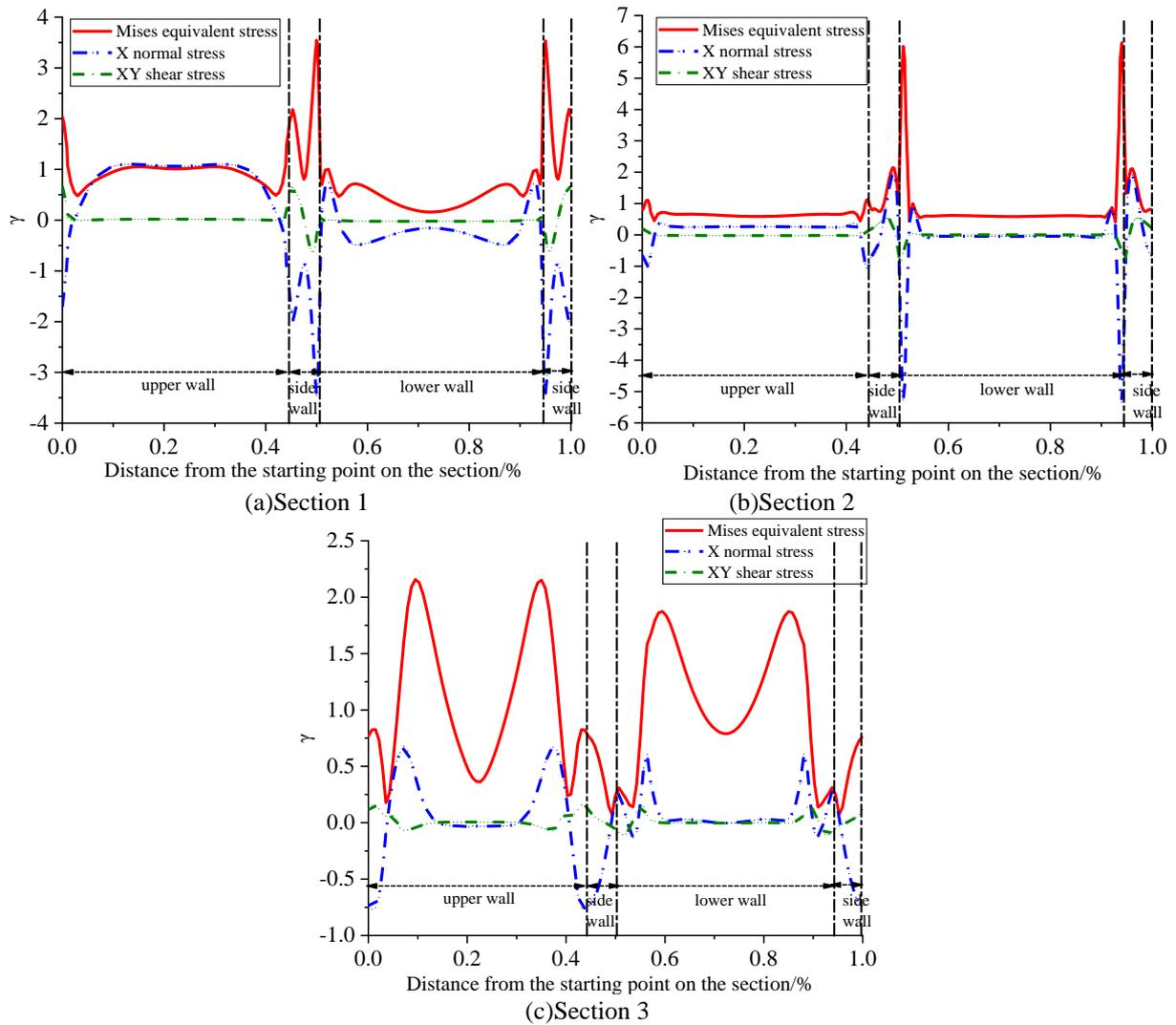
**Figure 6 Shear Lag Coefficient Curves on Three Characteristic Sections**
