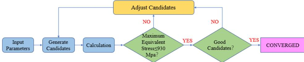
Figure 9 Optimization Workflow of Wall Thickness Distribution
