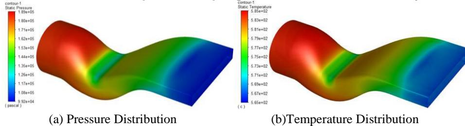
Figure 3 Flow Field Calculation of the Serpentine Nozzle
