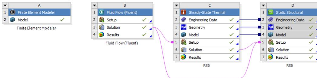
Figure2 Flow-Heat-Solid Sequence Coupling Calculation Process in Ansys Workbench
