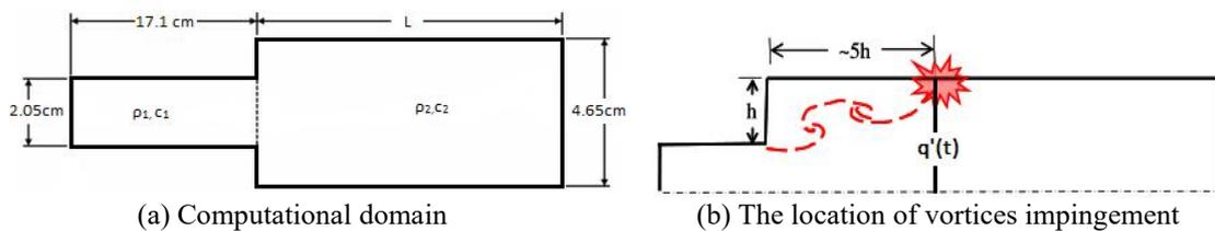
**Figure 8 Computational domain of experimental rig and the location of vortices impingement**
