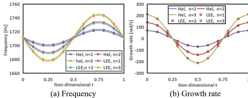
**Figure2 Variation of frequency and growth rate of 2L mode with  $n$  and  $t$**
