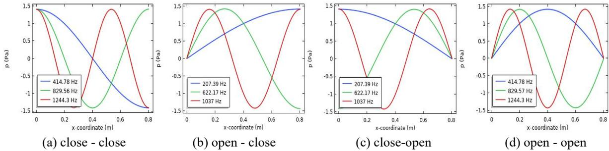
**Figure 1 first three order mode shapes of straight duct under various boundary conditions**
