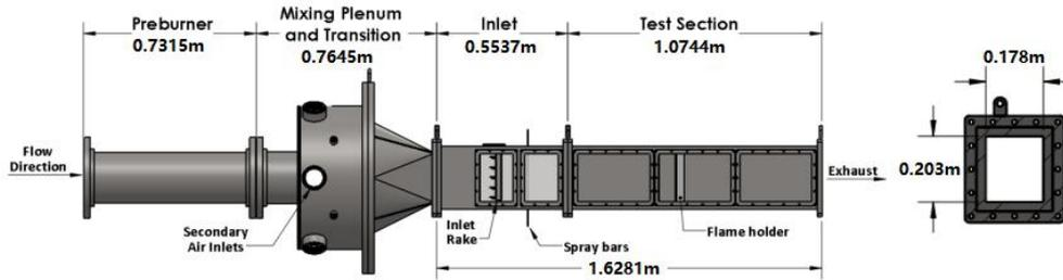
**Figure 3 Combustion Wind Tunnel Facility (Shaw et al., 2018)**
