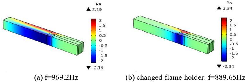
**Figure 6 Acoustic pressure for the first transverse modes along the width with temperature gradient**
