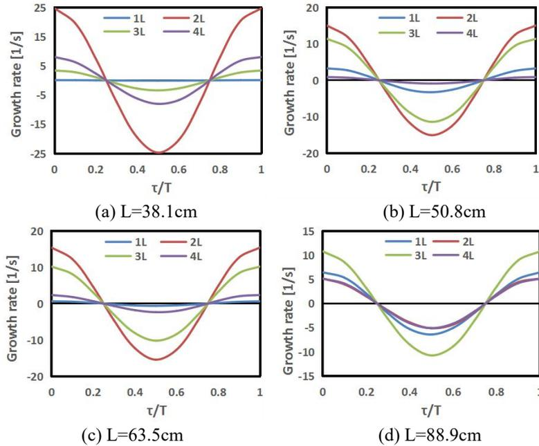
**Figure 9 The variation of growth rates of first 4L mode for different combustor length with  $n=1$**
