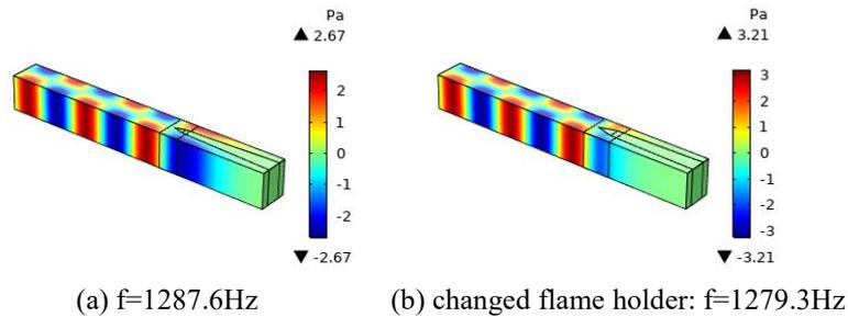
**Figure 7 Mode transition with temperature gradient**
