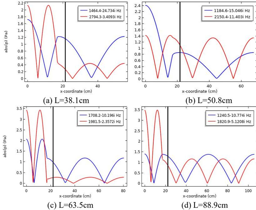
Figure 11 Acoustic pressure distribution in the combustion chamber
