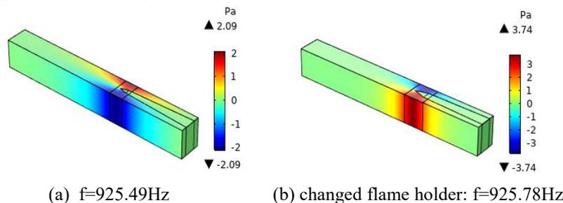
**Figure 5 Acoustic pressure for the first transverse modes along the width with flame holder**
