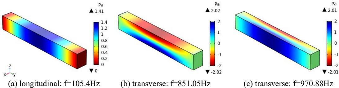
**Figure 4 Acoustic pressure for the first modes of rectangular tube**
