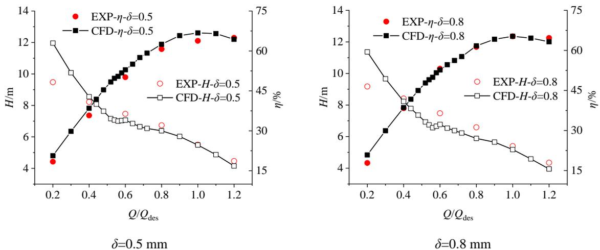
Figure 4 Comparison of external characteristic between numerical simulation and test
