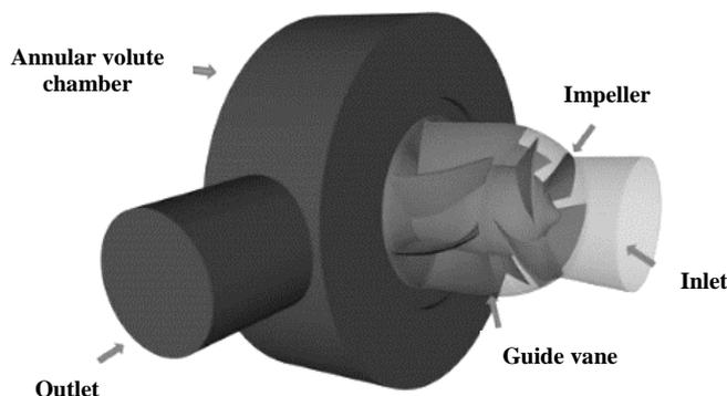
Figure 1 Mixed-flow pump 3D model
