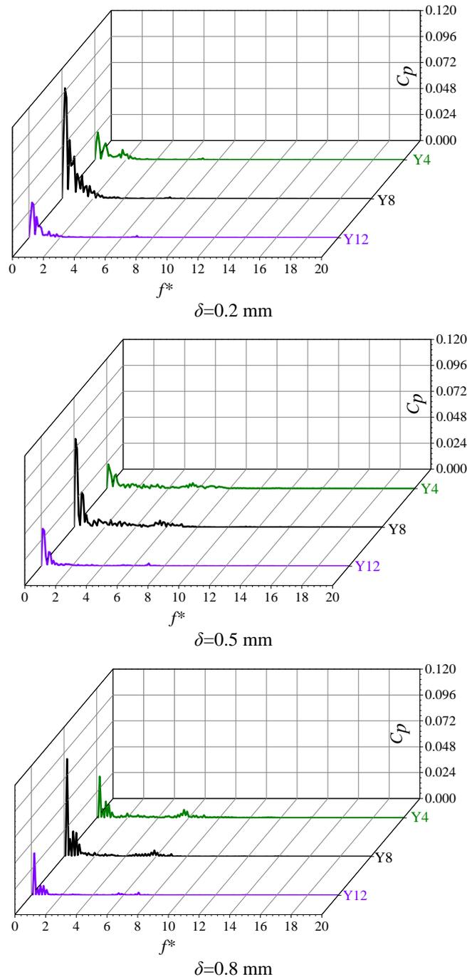
Figure 8 Frequency domain characteristics of pressure coefficient at Y4, Y8, Y12
