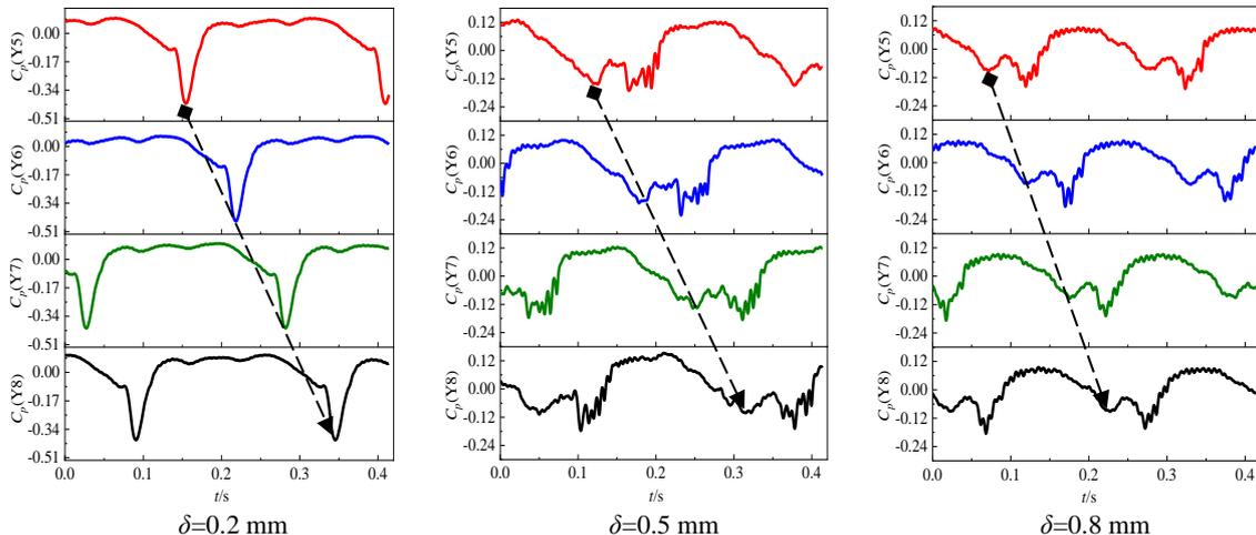
**Figure 6 Time-domain characteristics of pressure coefficient at Y5, Y6, Y7, Y8**
