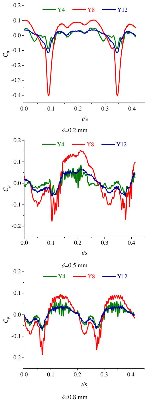
**Figure 7 Time-domain characteristics of pressure coefficient at Y4, Y8, Y12**
