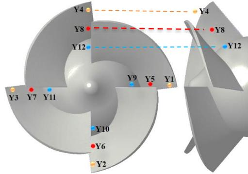
**Figure 5 Position of impeller outlet monitoring points**
