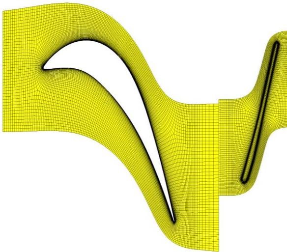
**Figure 2 Grid Diagram of Last Stage Blade**
