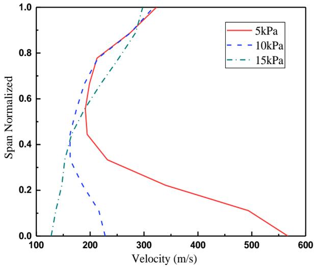
**Figure 6 Velocity Distribution at 50% Axial Section**
