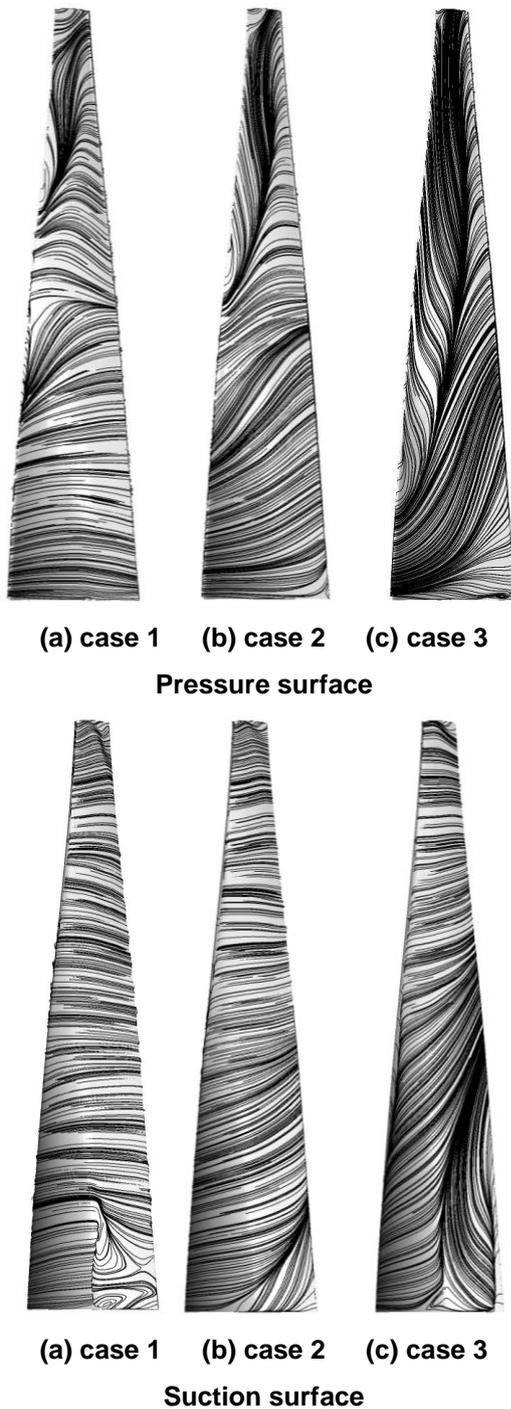
**Figure 4 Limit Flow Diagram of Rotor Blade Surface**
