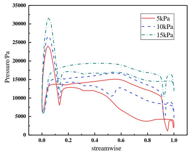
**Figure 5 Influence of Outlet Pressure on Tip Pressure**
