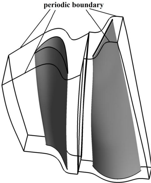
**Figure 1 Final Stage Model of Steam Turbine**
