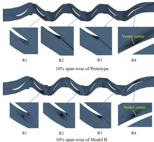
**Figure 5 Comparisons of limiting streamlines of prototype and model B**
