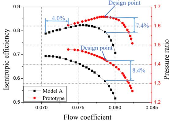
**Figure 2 Performance comparison between prototype and mode A**
