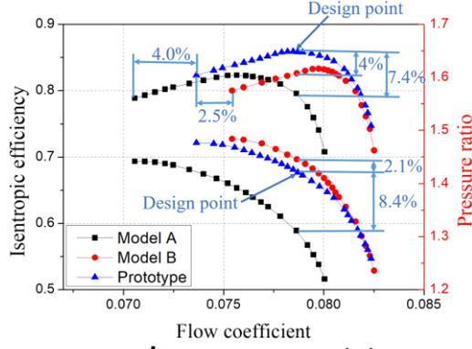
**Figure 3 Performance comparison among prototype, model A and model B**
