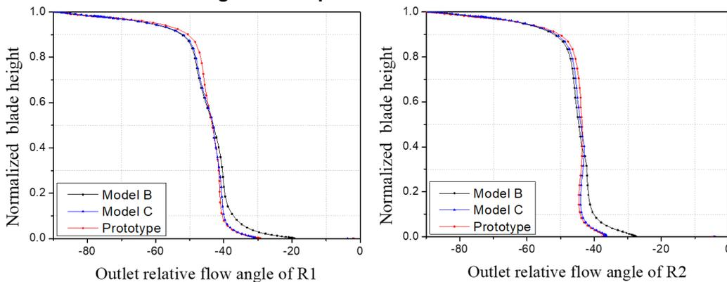
**Figure 7 Comparisons of outlet relative flow angle**
