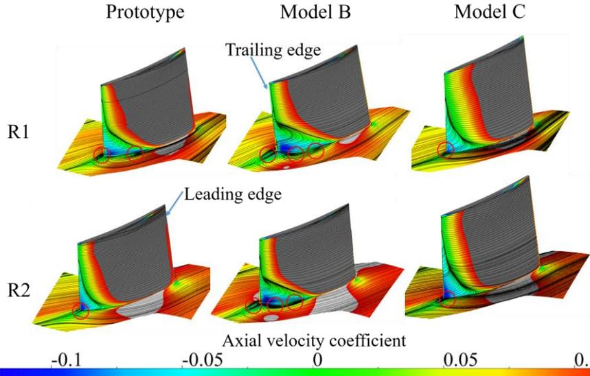
**Figure 8 Comparisons of flow fields among prototype, model B and model C**
