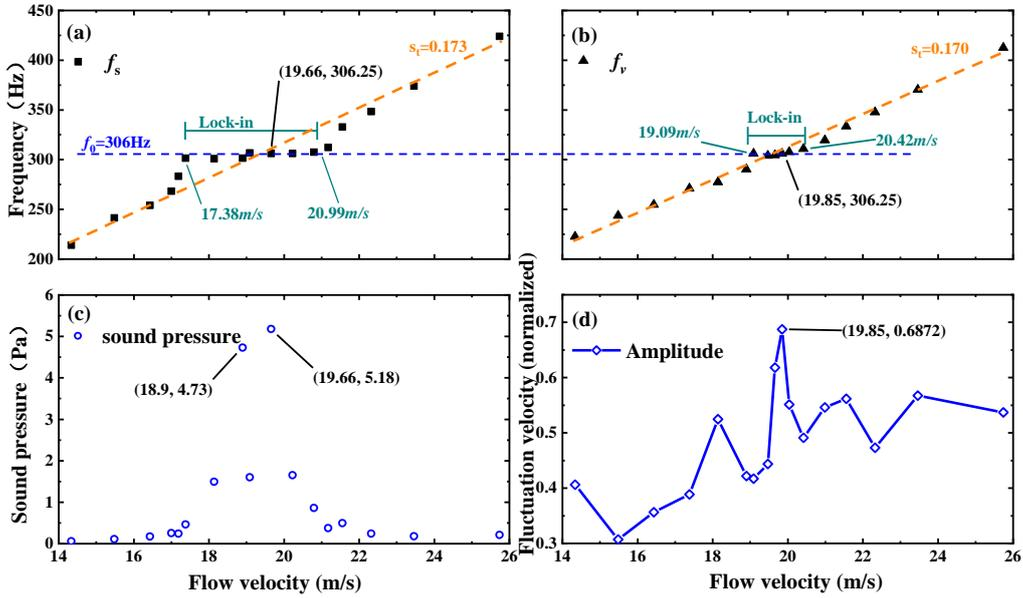
**Figure 3** The flow and sound field results in acoustic resonance: (a) frequency of sound field, (b) frequency of flow field, (c) sound pressure detected by microphone, (d) fluctuation velocity of vortex shedding
