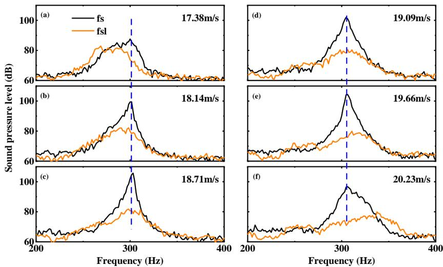
**Figure 11** Sound pressure level spectrum of lock-in region with acoustic liner
