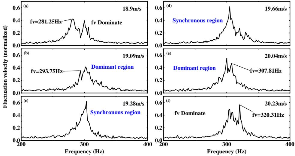
Figure 7 Vortex shedding spectrum of lock-in region with flow velocity
