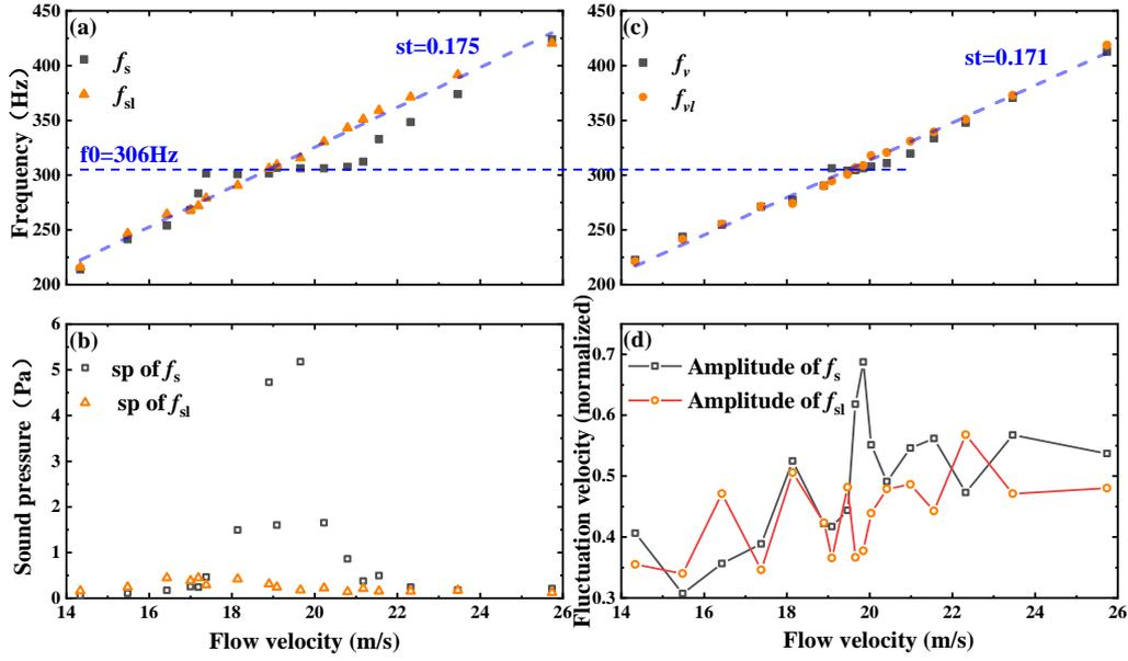
**Figure 10** The flow and sound field results in with acoustic resonance: (a) frequency of sound field, (b) frequency of flow field, (c) sound pressure detected by microphone, (d) fluctuation velocity of vortex shedding
