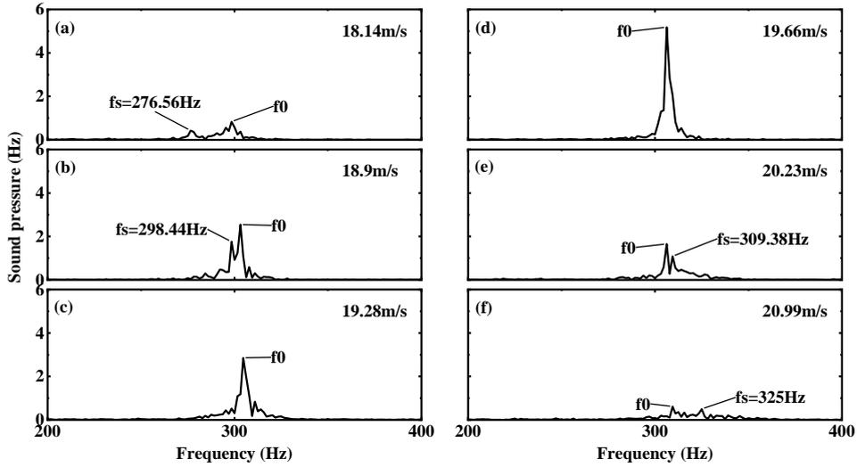
Figure 5 Sound pressure spectrum of lock-in region with flow velocity
