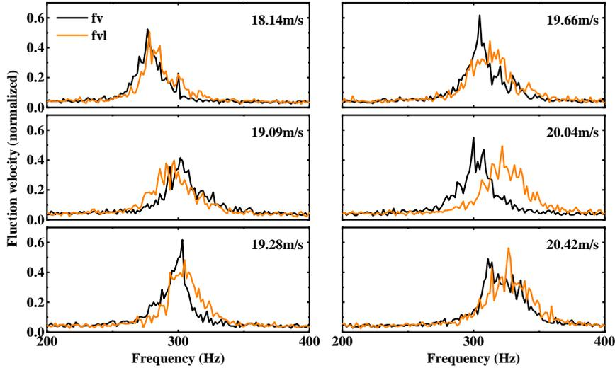
Figure 12 Vortex shedding spectrum of dominant region and synchronous region with acoustic liner
