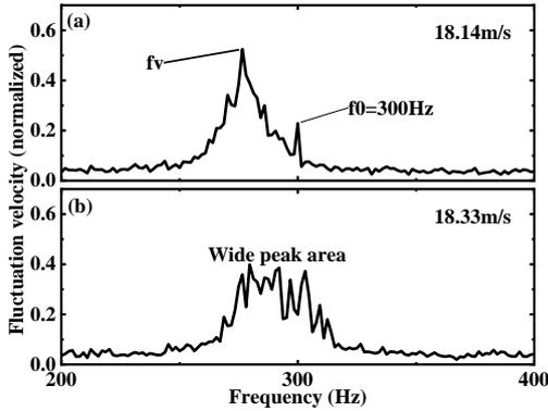
Figure 8 Spectrum of vortex shedding when  $u=18.14\text{m/s}$  and  $u=18.33\text{m/s}$
