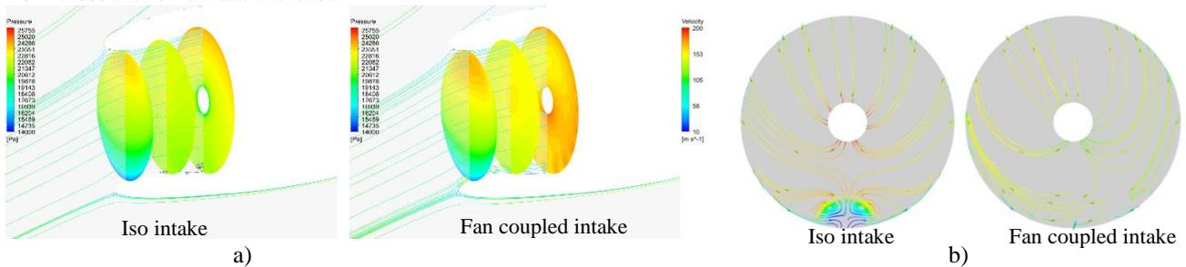
**Figure 12 Isolated intake and fan coupled intake comparison under cruise condition**
