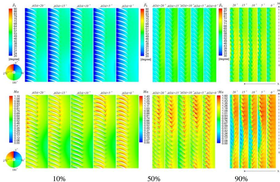
**Figure 14 blade to blade absolute flow angle and Ma distribution on different normalized span**
