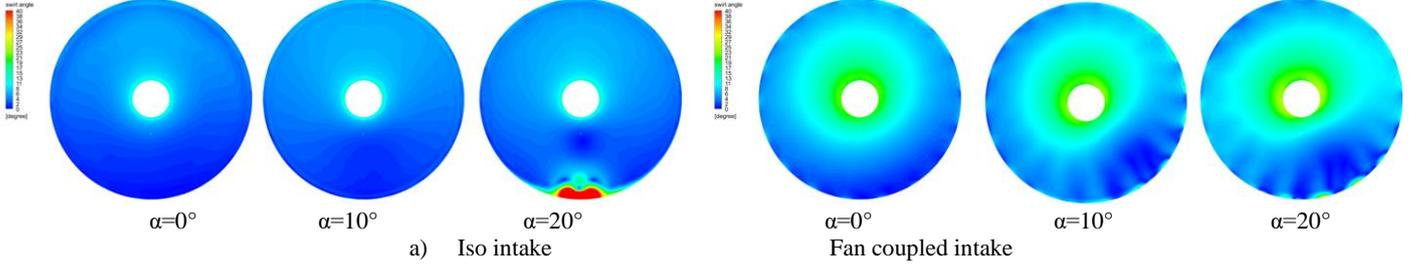
**Figure 15 Velocity angle contour on the inlet face of fan at cruise**
