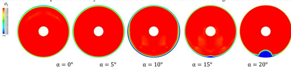
**Figure 9 Total pressure recovery coefficient distribution on AIP of isolated nacelle intake under cruise**
