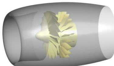
Figure 3 Nacelle intake and fan couple model
