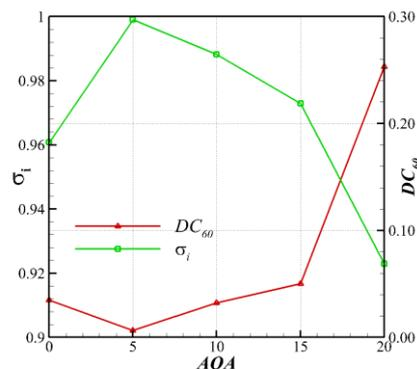
**Figure 10 Performance of the isolated nacelle intake vary with the AOA under cruise**
