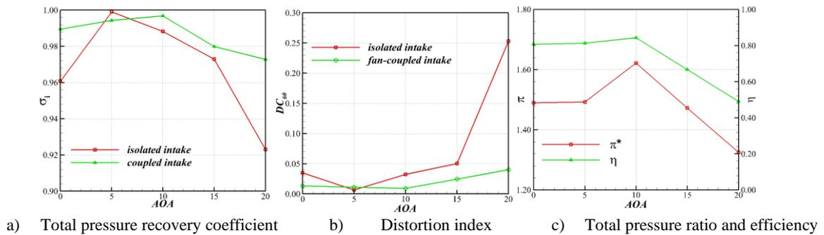
**Figure.11 Nacelle intake and fan performance under different AOA at cruise**
