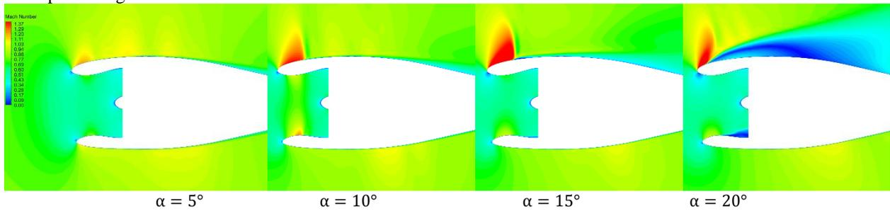
**Figure 8 Ma contour on the symmetry plane of the isolated nacelle intake under cruise**
