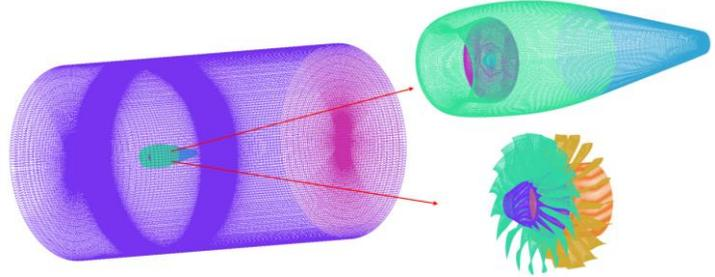
Figure 5 Grid of nacelle intake and fan blades
