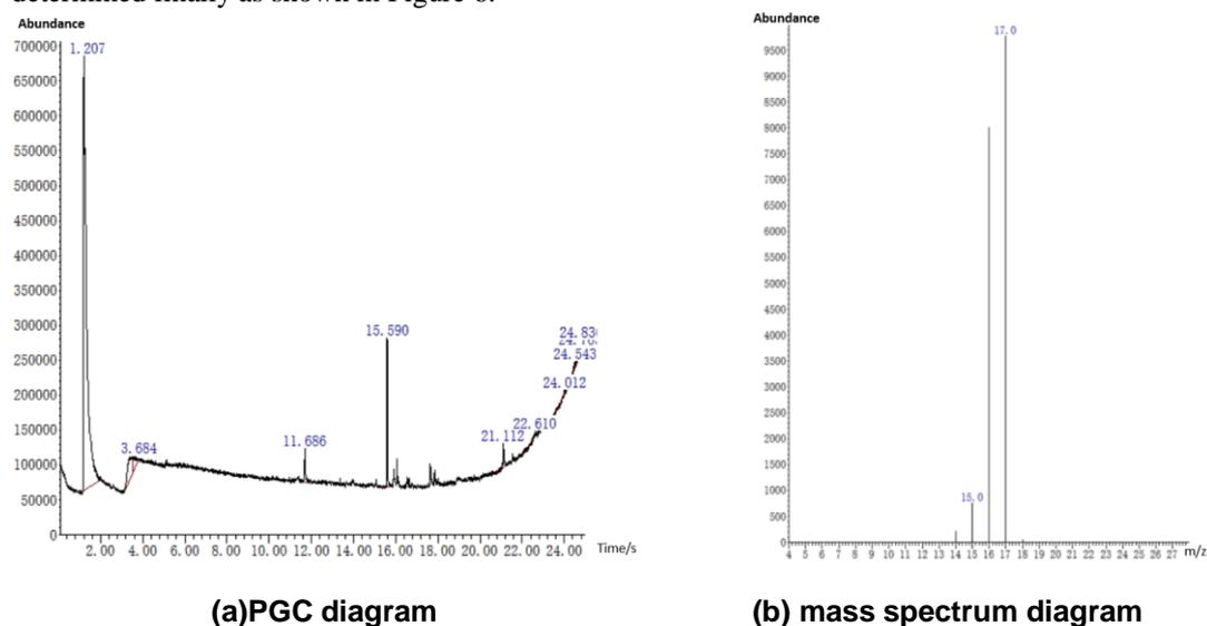
Figure 5 PGC and mass diagram of thermal cracking at 300°C
