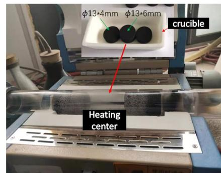
Figure 2 tube furnace heating experiment
