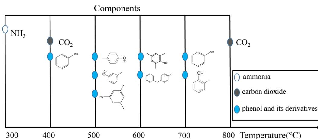
Figure 6 main components of gas at different temperatures in PY-GC-MS experiment
