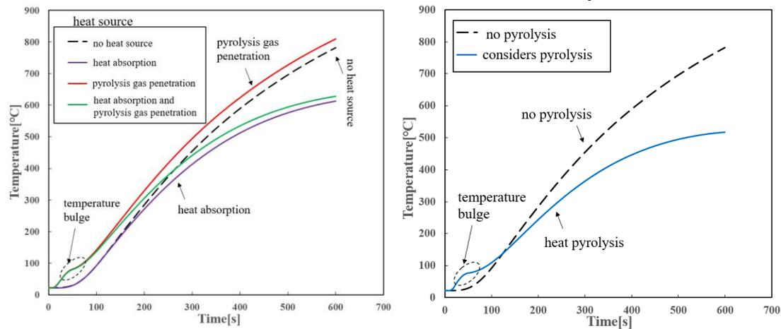
(c) the influence of extra heat source on the temperature change of outer wall surface
