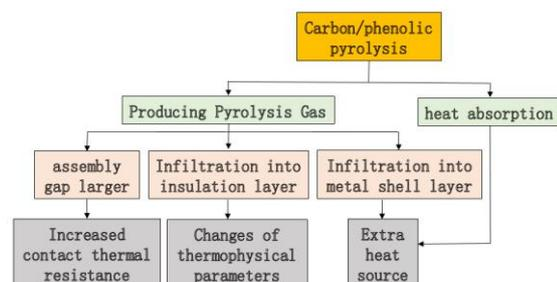
**Figure 4 Analysis of factors affecting thermal insulation performance by pyrolysis of carbon/phenolic materials**
