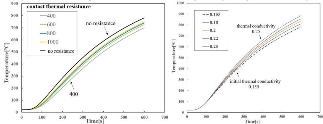
(a) the influence of contact thermal resistance on outer wall temperature
