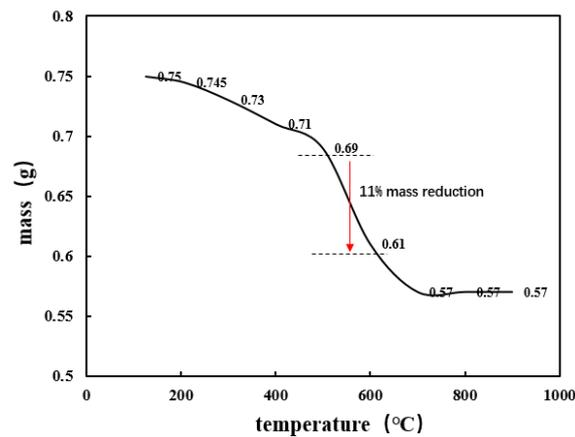
Figure 7 mass loss diagram of carbon/phenolic pyrolysis
