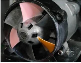
**Figure 4 The high-speed fan painted with PSP and TSP**
