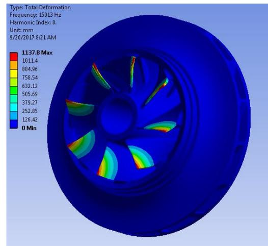
**Figure 11 The First Inducer Blade Mode of DMLS Impeller**
