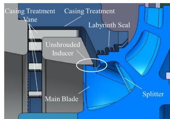
**Figure 1 Configuration of Novel Semi-shrouded Impeller with Casing Treatment**
