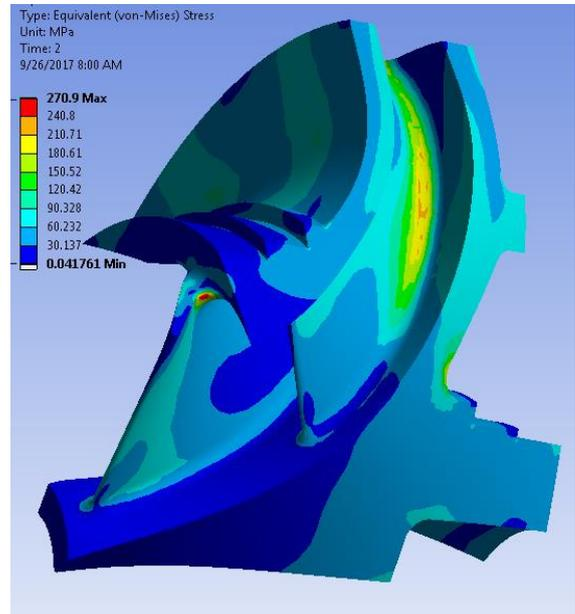
**Figure 10 Effective Stress of DMLS Impeller**
