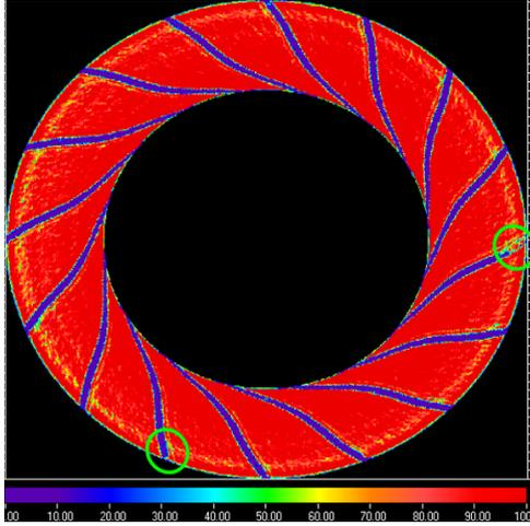
**Figure 3 UT scan of the Blade/Shroud Joint on an EBW Compressor Impeller**
