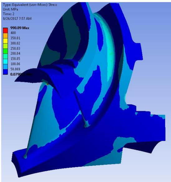
**Figure 9 Effective Stress of EBW Impeller**
