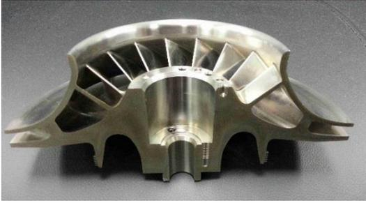
**Figure 5 Section Cut of DMLS Compressor**
