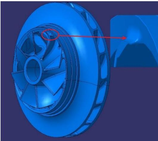
**Figure 6 DMLS Impeller with Inducer Unshrouded**
