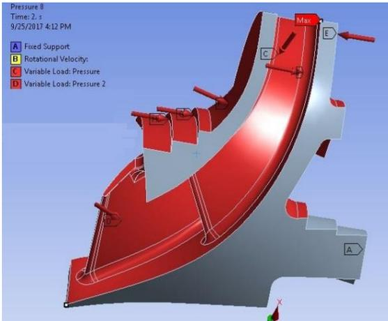
**Figure 8 Boundary Conditions of the FEA Model**
