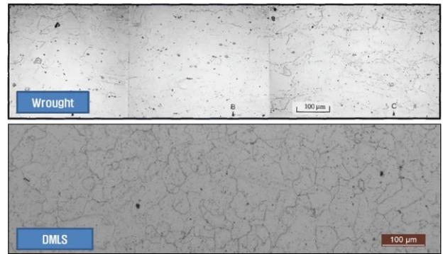
**Figure 4 Microstructure of Wrought and DMLS Material**
