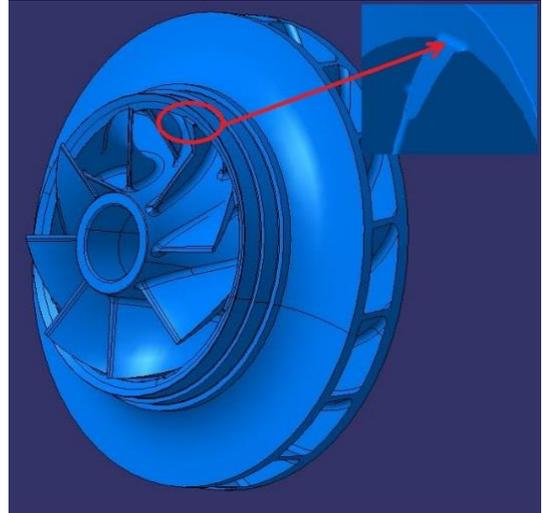
**Figure 7 EBW Semi-shrouded Impeller with 0.5mm Fillet Joint**
