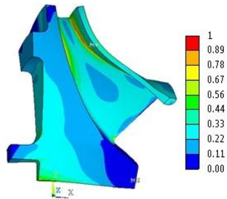
**Figure 2 Normalized Effective Stress of a Selected Compressor Impeller**
