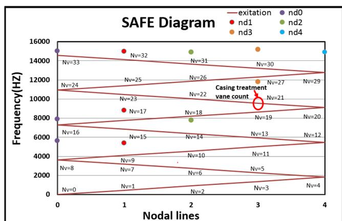
**Figure 12 SAFE Diagram of DMLS Impeller**
