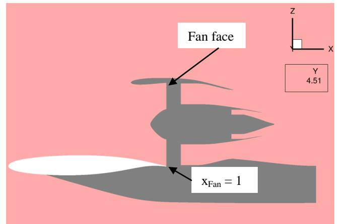
**Figure 2 Cross section through embedded propulsor at  $\eta = 0.31$**
