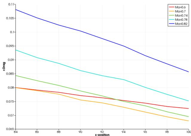
Figure 12 Drag coefficient  $C_D$  over engine position for different Ma numbers
