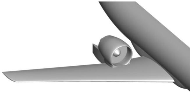
**Figure 3 View on embedded nacelle**
