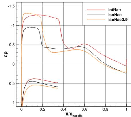
Figure 10  $c_p$  distribution of isolated and integrated nacelle at 12o'clock for  $x_{Fan} = 1$
