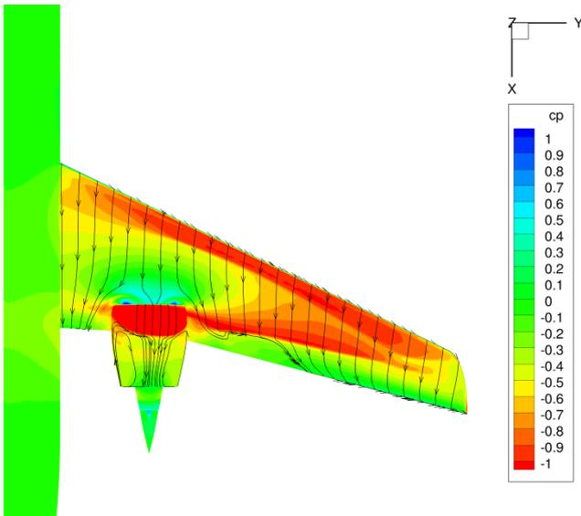
**Figure 7 Isobars and skin friction lines of WBE with engine at  $x_{Fan} = 1$**
