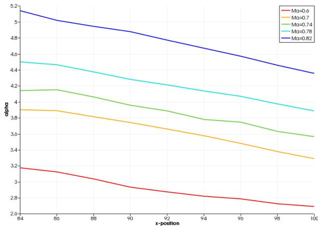
Figure 11 Angle of attack over engine position for different Ma numbers
