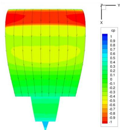
**Figure 5 Isobars of isolated nacelle (view on the 12 o'clock section)**
