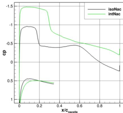
Figure 9  $c_p$  distribution of isolated and integrated nacelle at 12o'clock for  $x_{Fan} = 0.84$
