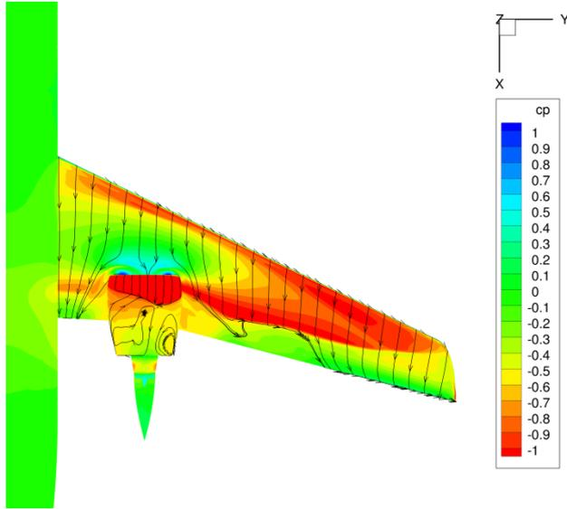
**Figure 6 Isobars and skin friction lines of WBE with engine at  $x_{Fan} = 0.84$**
