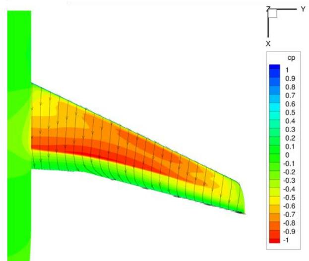
**Figure 4 Pressure isobars on upper wing surface for  $Ma = 0.78$**
