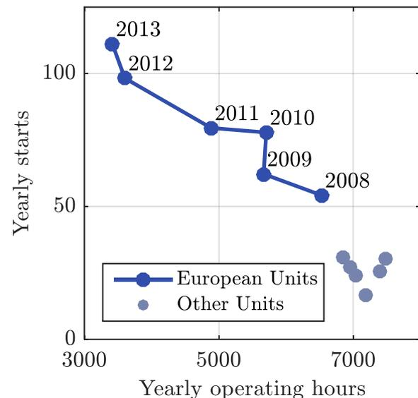
**Figure 1: European and Non-European gas turbine units of the former Alstom GT24/GT26 fleet show different operation regime. Figure reproduced from [1].**
