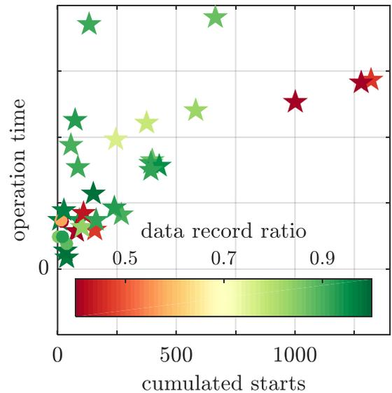
**Figure 3: Fleet investigation on (partial) independence of starts and operating hours (Round points show insufficient total interval time or drift data points).**
