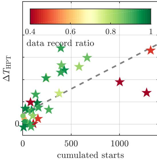
**Figure 6: Operation time averaged HPT outlet measurement drift vs. engine starts per day of available data logging (Round points show insufficient total interval time or drift data points).**
