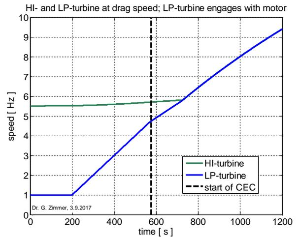
**Figure 16 Engagement while both steam turbine sections are at drag speed**
