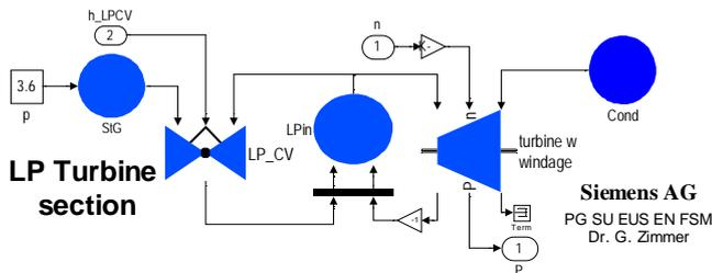
Figure 7 Thermodynamic model of the LP turbine
