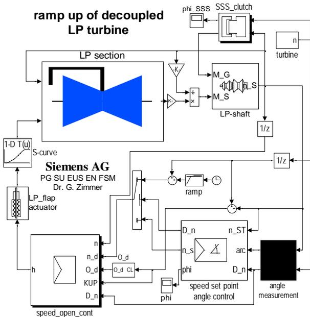
**Figure 8 Overall simulation model (LP and HP/IP section engaged at nominal speed)**
