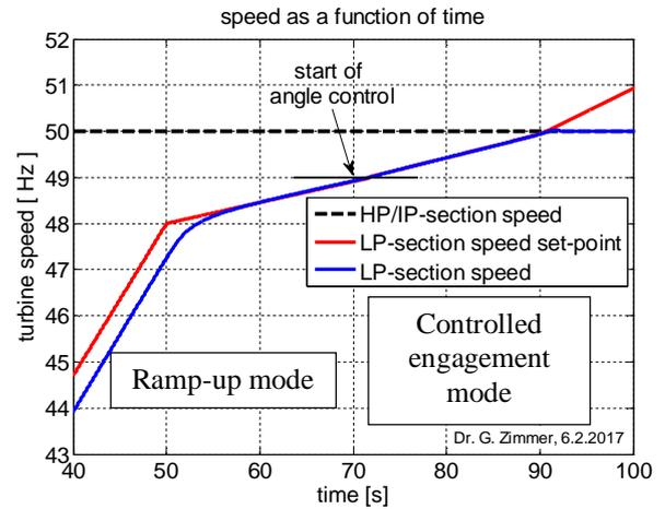
**Figure 9 Speed set-point and actual speed (simulation) for the LP turbine at ramp-up**
