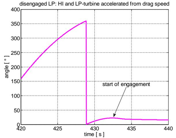
**Figure 15 Angle difference at start of engagement from HP/IP-coast down, target angle is 0°**
