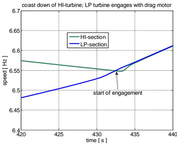
**Figure 14 Engagement while HP/IP turbine coasts down; detail at start of engagement**
