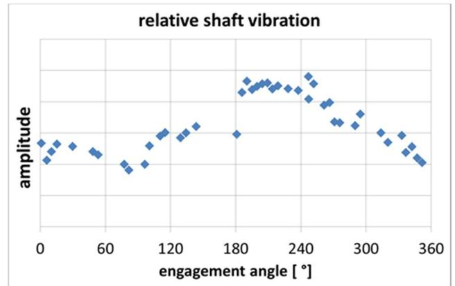
**Figure 4 Relative shaft vibration for different engagement angles**
