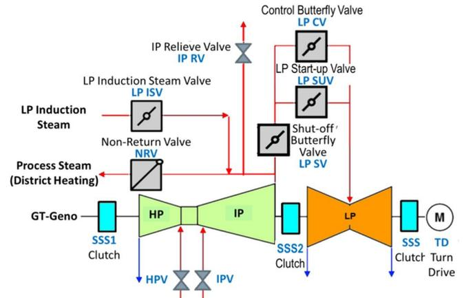
**Figure 3 Configuration detail**
