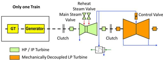
**Figure 2 Single-shaft CHP turbine train configuration with one extraction**
