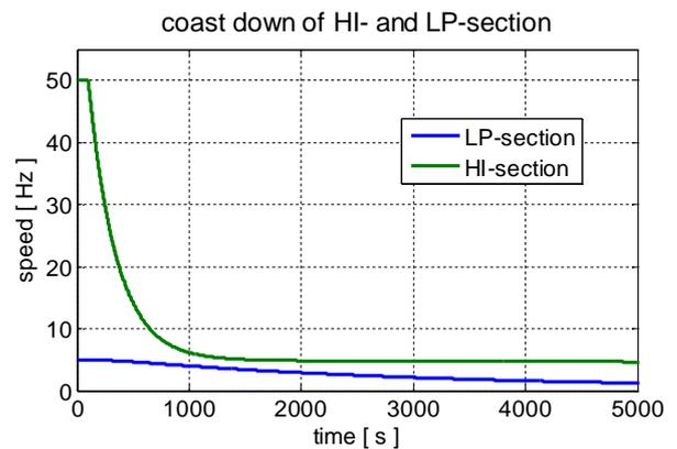
**Figure 12 Drag speed of LP- and HP/IP turbine**
