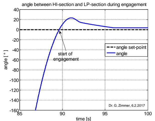
**Figure 10 Angle between HP/IP- and LP section prior to engagement; set-point is 0°**
