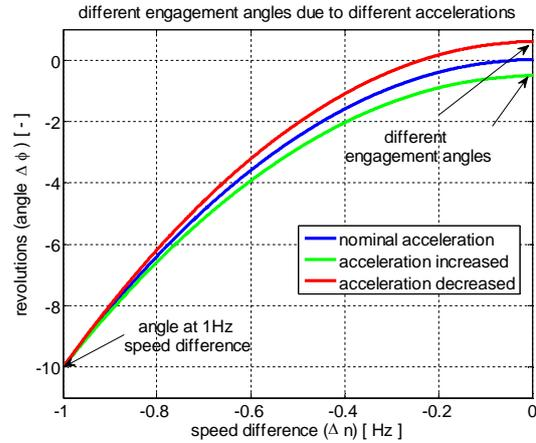
Figure 5 Dependency of clutch engagement angle on chosen acceleration
