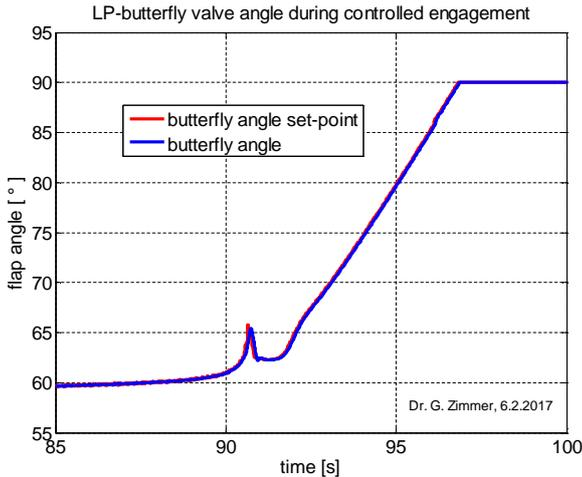
**Figure 11 Angle of LP butterfly control valve prior to engagement; possible maximum is 90°**
