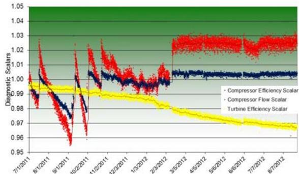
Figure 5: Mercury 50 Field Data Component Diagnostic Scalars
