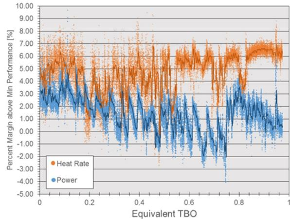
Figure 6: Titan 250 Field Data Heat Rate and Power Margin
