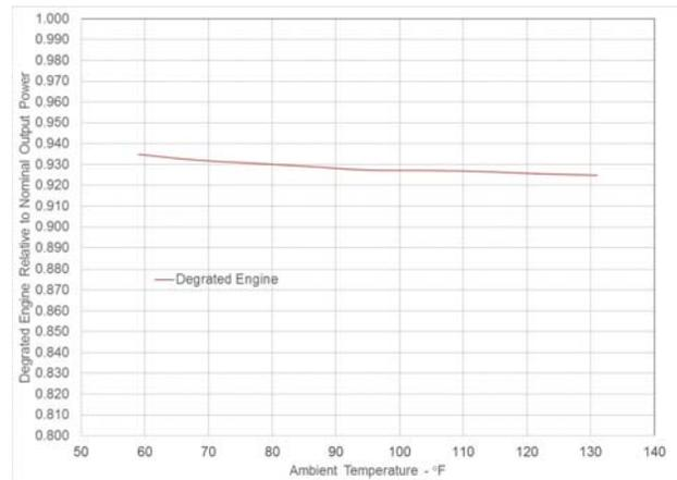
Figure 11: Titan 250 Normalized Power, Effect of Comp Degradation
