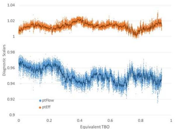
Figure 9: Titan 250 Field Data PT Turbine Diagnostic Scalars
