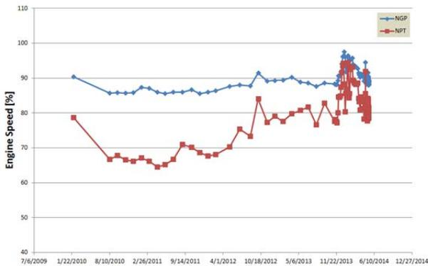
Figure 12: Mars 100 Field Data Engine Speeds to TBO
