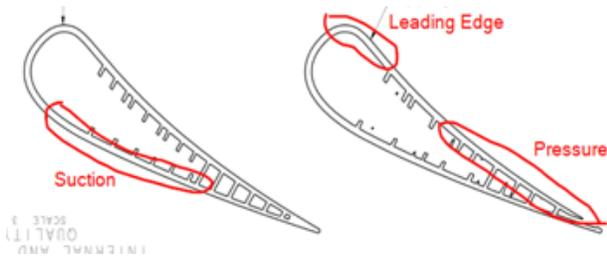
Figure 13: Airfoil Locations of Surface Finish Measurements
