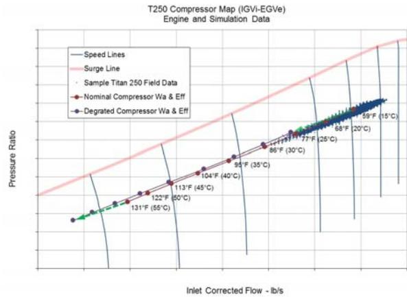
Figure 10: Titan 250 Compressor Map with Field and Simulation Data
