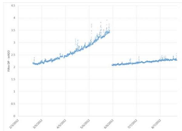
Figure 3: Mercury 50 Field Data Inlet Filter DP
