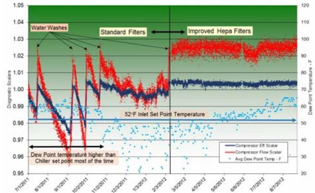
Figure 2: Mercury 50 Field Data Recoverable Compressor Degradation
