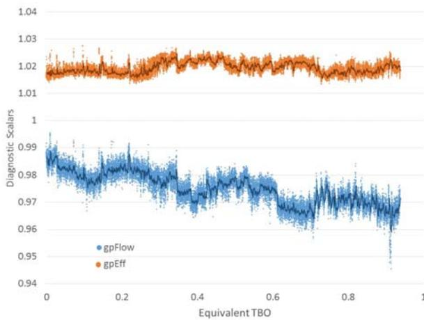
Figure 8: Titan 250 Field Data GP Turbine Diagnostic Scalars
