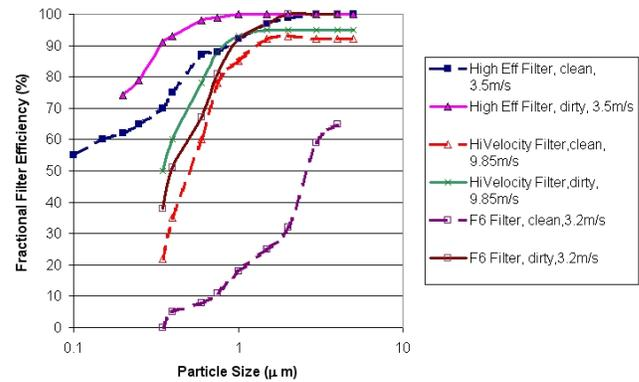
Figure 1: Comparison of fractional efficiency for filter elements from different suppliers and different face velocities in new and dirty conditions [12].
