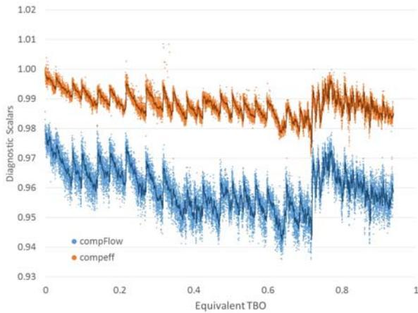
Figure 7: Titan 250 Field Data Compressor Diagnostic Scalars
