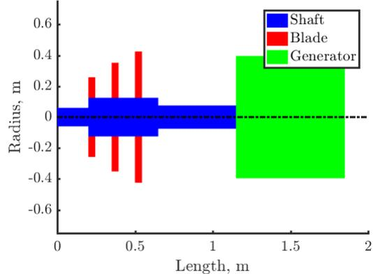
**FIGURE 6:** Sketch of the rotor model
