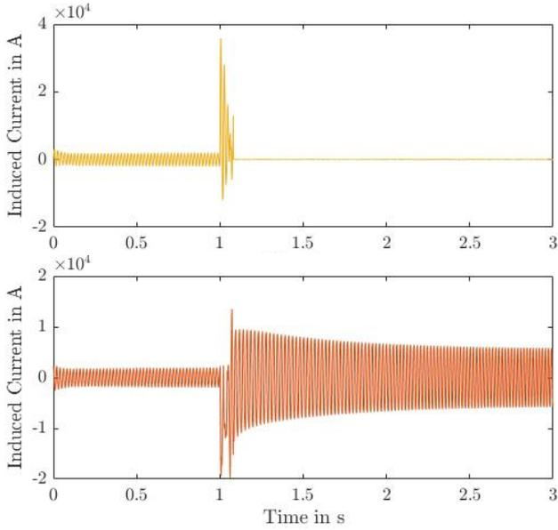
**FIGURE 7:** Currents induced in line 3 without short (top) and line 2 (bottom), which is shorted to line 1
