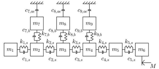
FIGURE 1: Lumped-mass model of the rotor
