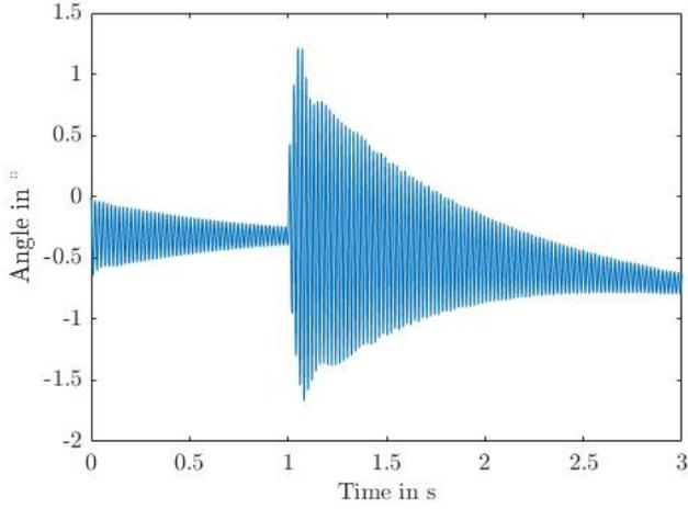
**FIGURE 8:** Response of the last stage to a two-pole short circuit
