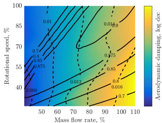
FIGURE 2: Aerodynamic damping (log dec) for ND 0, solid lines show isentropic efficiency
