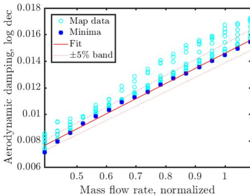
**FIGURE 3:** Aerodynamic damping (log dec) over mass flow rate, solid line represents a linear fit of the respective minima
