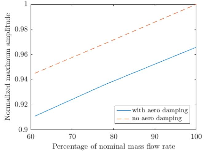
**FIGURE 10:** Normalized maximum response amplitude with and without aerodynamic damping
