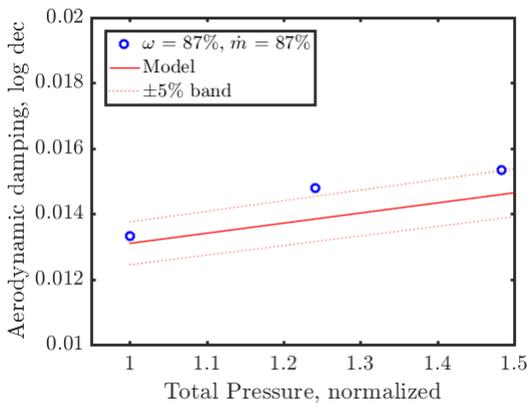
**FIGURE 5:** Comparison of the damping model (Eq. 5) with CFD results for operating point  $\omega = 87\%$ ,  $\dot{m} = 87\%$
