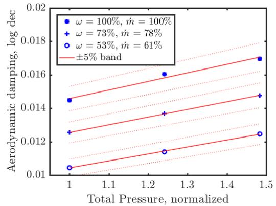
**FIGURE 4:** Aerodynamic damping (log dec) for higher total pressure levels
