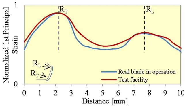
**Figure 9: Strain distribution in the test facility compared to real operation**
