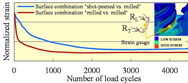
**Figure 17: Measured strains under LCF loading**
