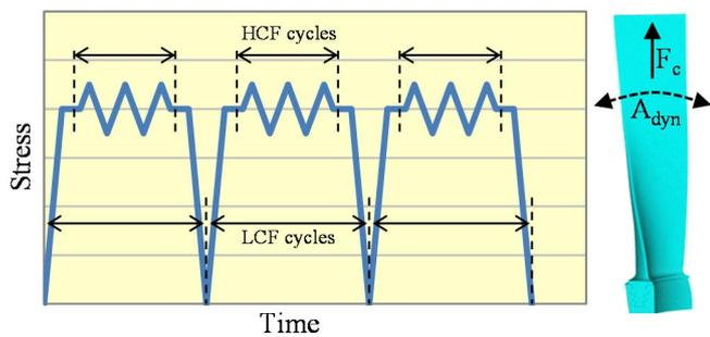
**Figure 1: Typical loading conditions of LP blades**
