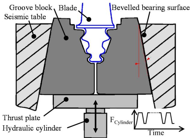
**Figure 3: Clamping device**
