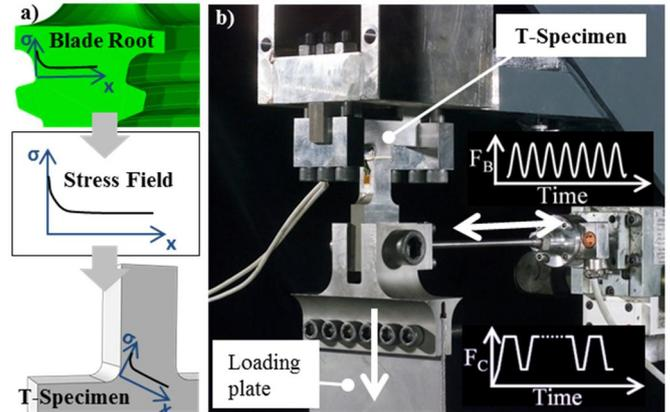
**Figure 2: a) Testing principle b) Testing facility for small-scale T-specimens [1]**
