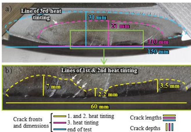
**Figure 13: Crack surface analyses a) Fracture surface b) Crack initiation area**
