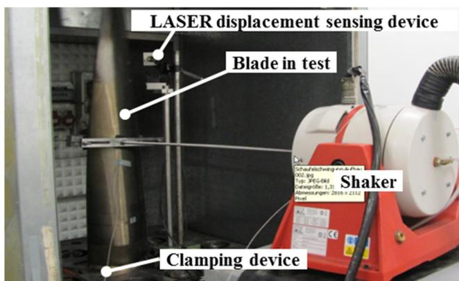
**Figure 4: HCF component test facility**
