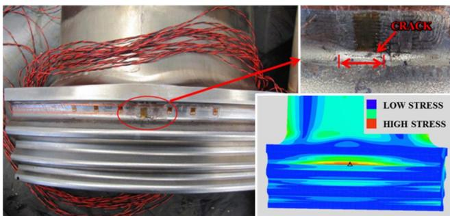
**Figure 10: Crack initiation location of tested blade compared to prediction**
