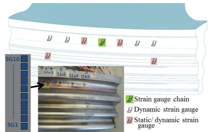
**Figure 5: Location of strain gauges at suction side**
