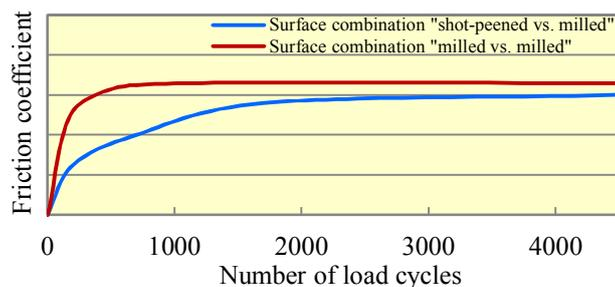
**Figure 18: Friction coefficients under LCF loading**
