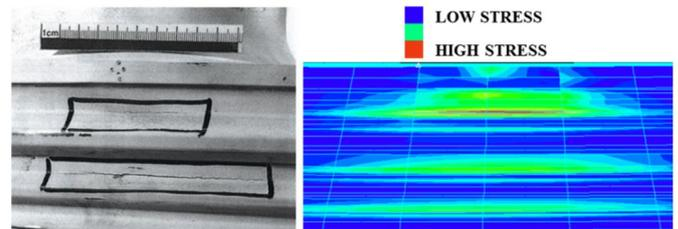
**Figure 15: Crack initiation location of a tested blade compared to prediction**
