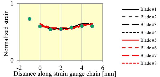
**Figure 19: Comparison of measurement and FE results along the strain gauge chain**
