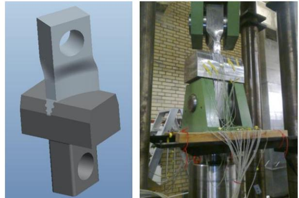
**Figure 8: 3D model and test facility for blade-to-rotor connection investigations**
