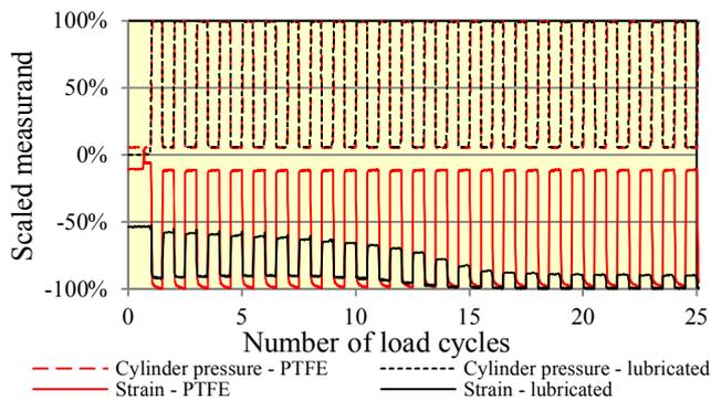
**Figure 6: Influence of lubrication on the relief behaviour**
