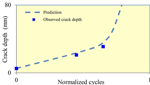
**Figure 14: Comparison of measured and predicted crack depths**
