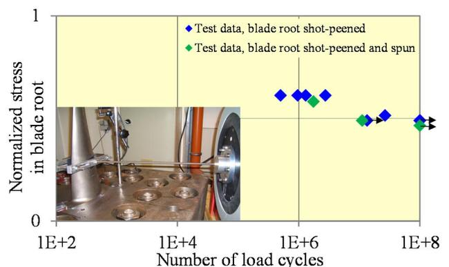
**Figure 12: Influence of spinning of shot-peened blades on the fatigue behavior**
