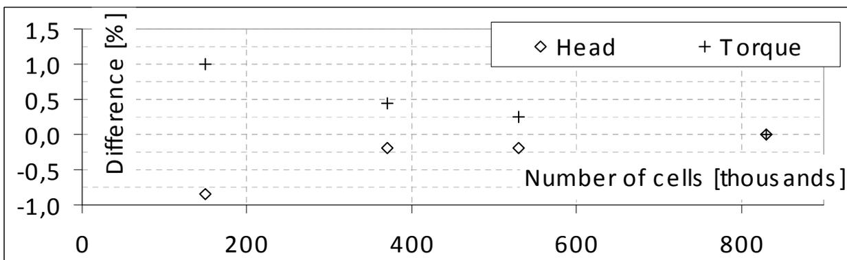
**Fig. 4: results of the grid dependence investigation. The relative difference in computed head and torque with reference to the simulation of the finest mesh resolution are plotted versus the mesh size, in thousands of cells [10].**
