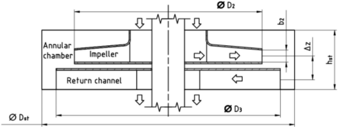
**Fig. 1: schematic representation of a meridional section of a generic stage. The impeller, one return channel and the annular chamber are indicated. The flow path of the main stream is represented by arrows. The main geometrical features of the stage are referenced.**
