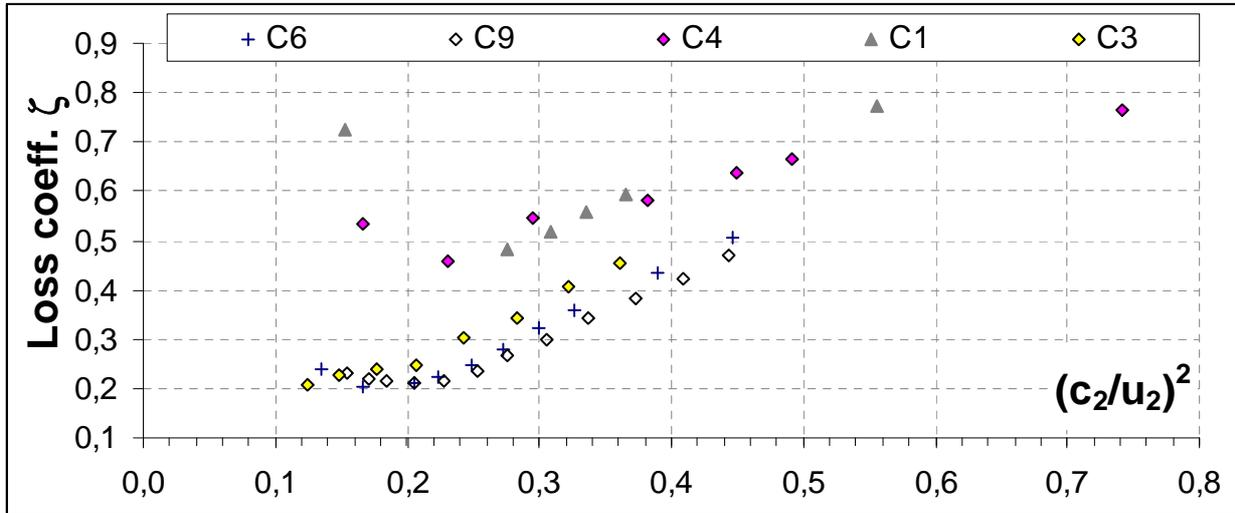
**Fig. 6: loss coefficient versus the dynamic head, made dimensionless according to the dynamic head corresponding to the blade tip velocity.**
