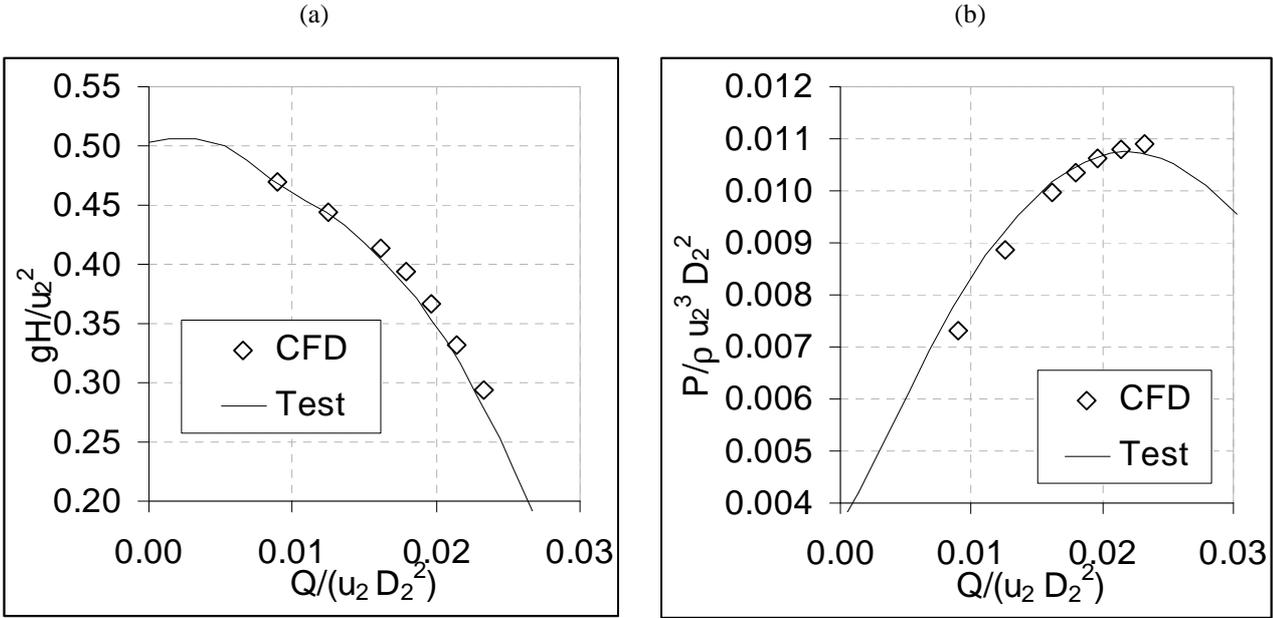
**Fig. 5: comparison between measurements (solid lines) and numerical results (empty markers): a) head per stage versus the flow rate, b) absorbed power per stage versus the flow rate. All quantities are presented in dimensionless form.**
