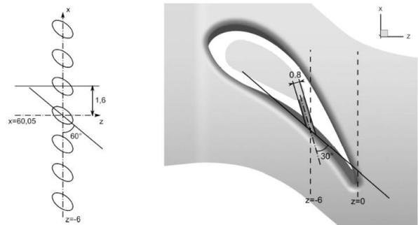
Figure 2 - Geometry of the vane cooling channels: meridional plane (left), tangential plane (right)
