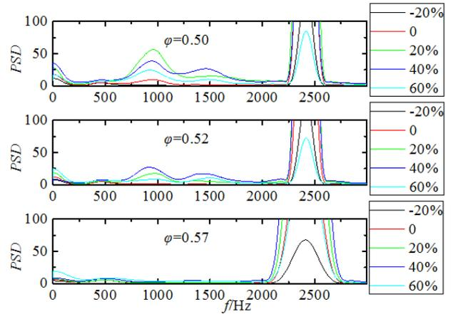
Fig.4 PSD results (2400 rpm, 1.1 mm)
