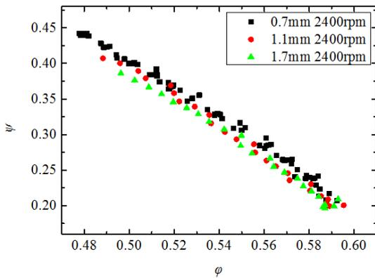
Fig.7 Compressor performance map at 2400 rpm
