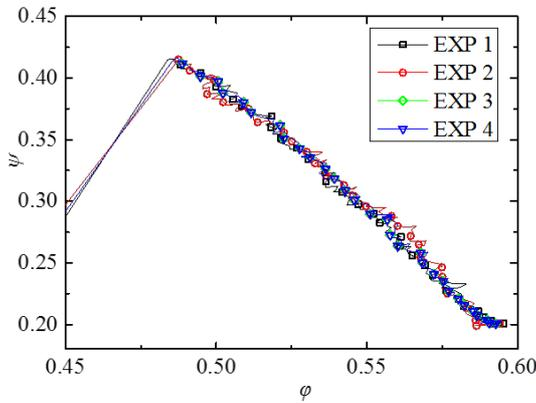
Fig.3 Compressor characteristic lines (2400 rpm, 1.1 mm)
