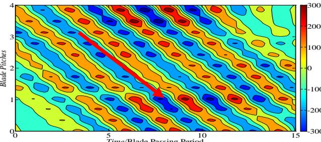
Fig.5 Time-space pressure contours (2400 rpm, 1.1 mm)
