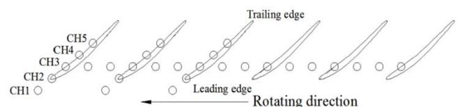
Fig.2 Arrangement of dynamic pressure sensors
