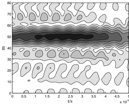
Fig.6 Mode orders at  $\phi = 0.49$  (2400 rpm, 1.1 mm)
