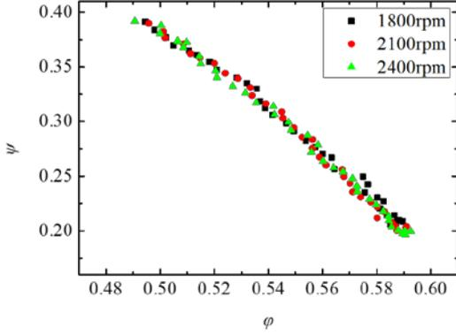
Fig.11 Compressor performance map with 1.7 mm tip clearance size
