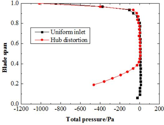
Fig.14 Radial profile of inlet total pressure
