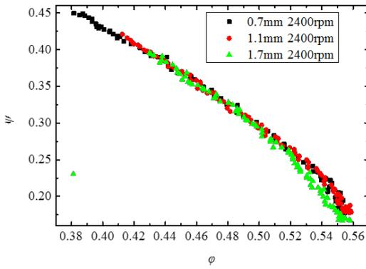
Fig.15 Compressor performance map at 2400 rpm
