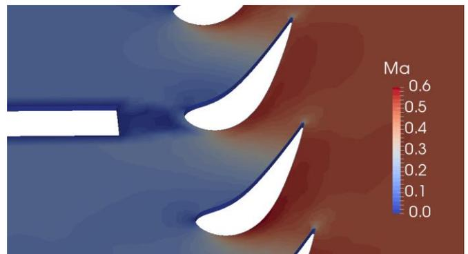
Figure 7 Mach number in the can gap area
