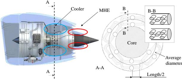
**FIGURE 8. Schematic of the modified GE90-94B turbofan engine showing the positioning of the cooler and the heater of the scCO<sub>2</sub> waste heat recovery unit and a simplified section and detail of the cooler.**
