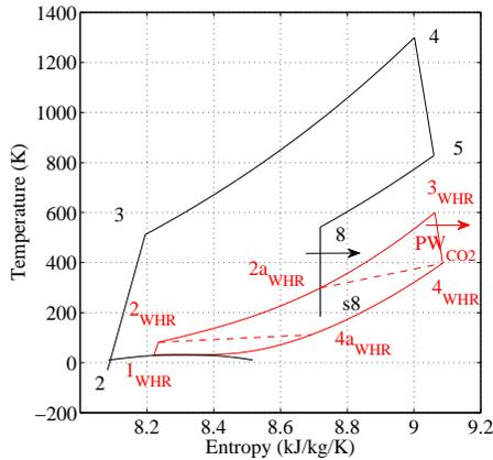
(b) Thermodynamic cycles in the  $T-s$  diagram of  $\text{CO}_2$ . The values of specific entropy of the state points related to the gas turbine engine cycle have been scaled appropriately in order to correctly correspond to the pertinent  $\text{scCO}_2$  cycle state points, thus neglecting that they refer to different working fluids.
