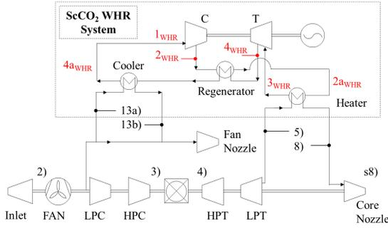
(a) Simplified process flow diagram
