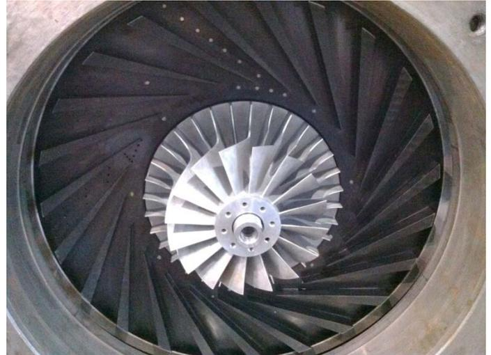
**Figure 4 A Photo of the Test Impeller and Transducers**
