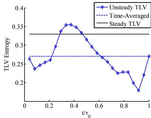
**Fig. 15 Unsteady Tip Leakage Generation, Normalized by Mixed Out Entropy Generation in 'SF' Case**
