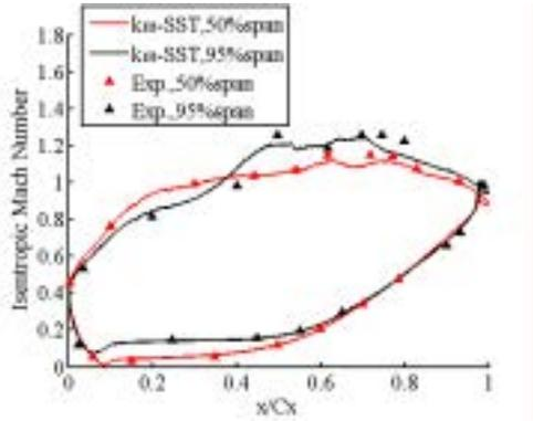
**Fig. 4 Isentropic Mach Number Distribution along the Blade Middle Span and Near the Tip Region (Experimental Data from Zhang et al. [26])**
