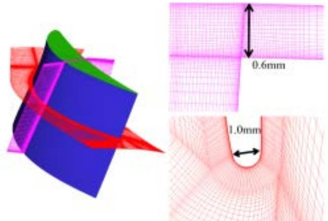
**Fig. 3 Mesh on the Cut Planes of 0.5Cx and Near Trailing Edge**
