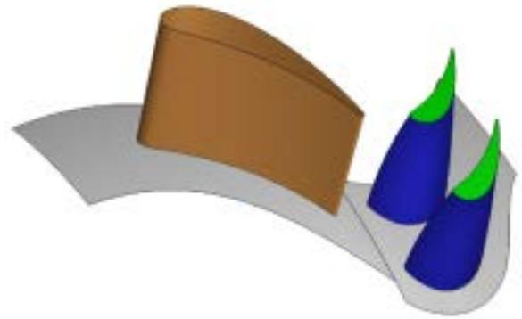
**Fig. 1 Computational Domain with a Rotor Flat Tip**
