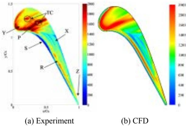
**Fig. 5 Heat Transfer Coefficient ( $W/m^2K$ ) on the Blade Tip by (a) Experiment (from Zhang et al.[26]) and (b) CFD**
