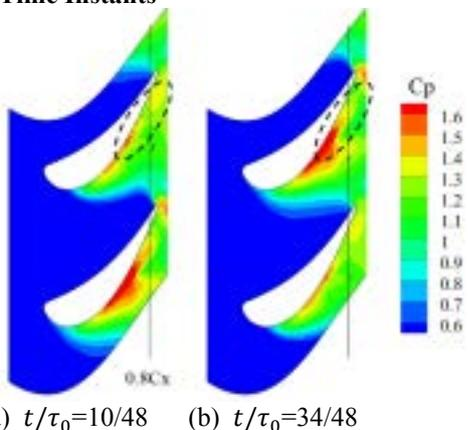
**Fig. 13 Static Pressure Coefficient on the Cut Plane of 95% Span for Two Time Instants**
