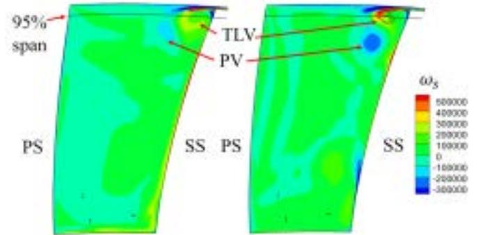
**Fig. 14 Streamwise Vorticity ( $\text{s}^{-1}$ ) on the Cut Plane of  $0.8C_x$  for Two Time Instants**
