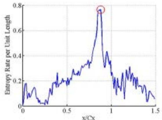
Fig. 9 Tip Leakage Loss per Unit Length ( $\text{JK}^{-1}$ ) Along Axial Direction
