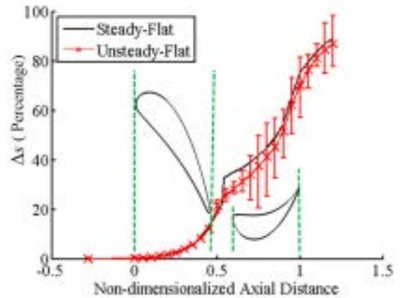
**Fig. 6 Entropy Variation along Axial Direction for 'SF' and 'UF', Normalized by the Mixed Out Entropy in 'SF'**
