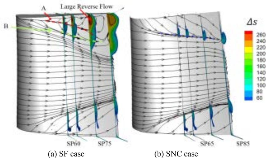
Fig. 7 Limiting Streamlines on Suction Surface and Entropy Rise ( $\text{Jkg}^{-1}\text{k}^{-1}$ ) for 'SF' and 'SNC'
