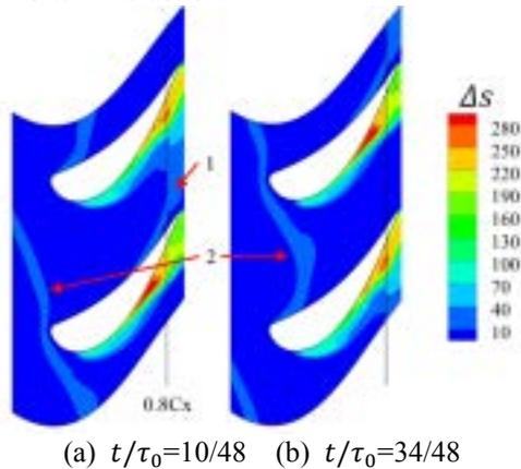
**Fig. 12 Entropy ( $\text{Jkg}^{-1}\text{K}^{-1}$ ) on the Cut Plane of 95% Span for Two Time Instants**
