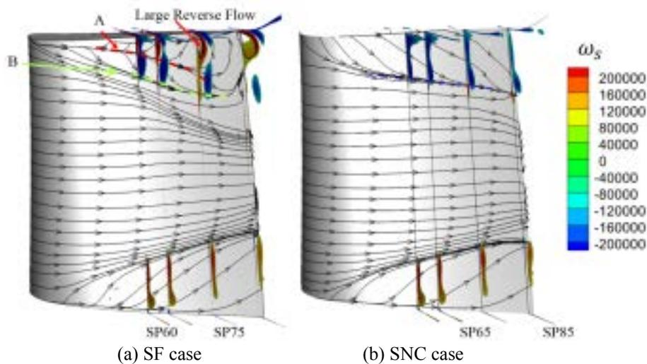
Fig. 8 Limiting Streamlines on Suction Surface and Streamwise Vorticity for 'SF' and 'SNC'
