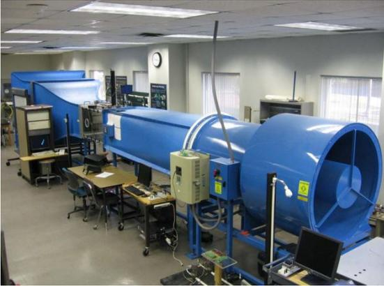
Figure 8. Baylor Subsonic Wind Tunnel
