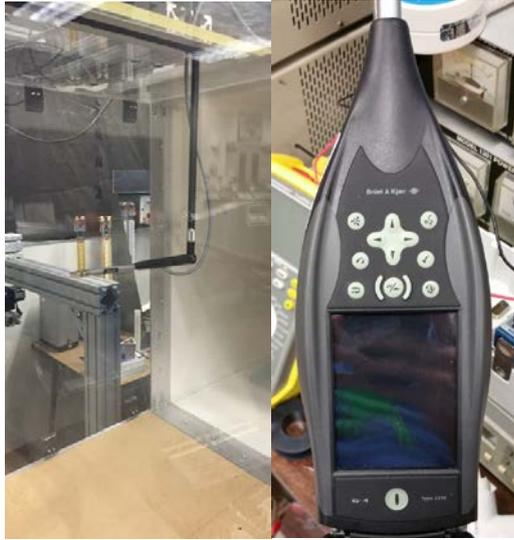
Figure 11. Brüel & Kjaer Microphone and Analyzer
