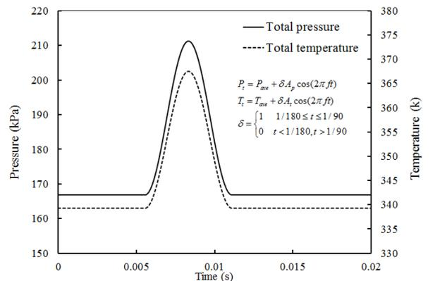
Figure 5. single pulse imposed at inlet of the turbine
