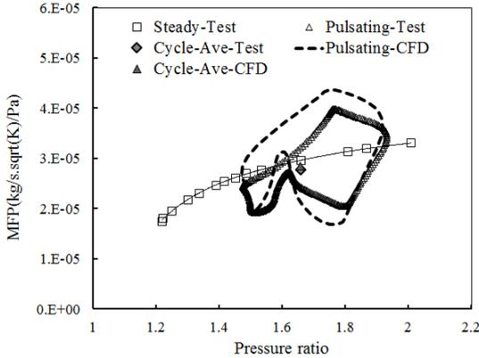
Figure 4. swallowing capacity at 60 Hz, middle load, 50 kRPM
