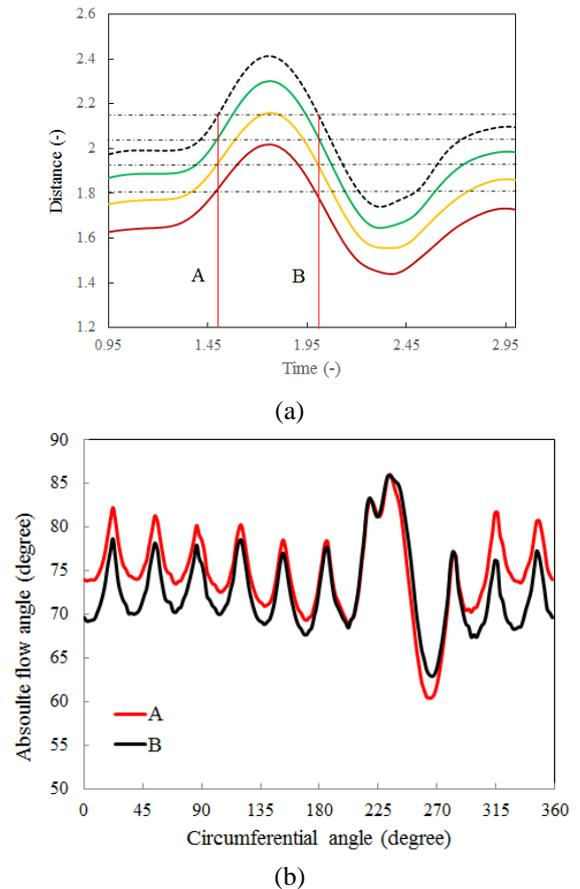
Figure 7 (a) two instant times with the same pressure at the rotor inlet; (b) absolute flow angle distributions in annulus at two instant times
