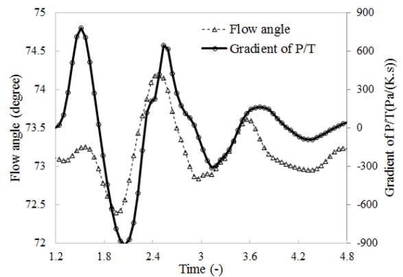
Figure 11 flow angle and the pressure gradient under the pulsating condition
