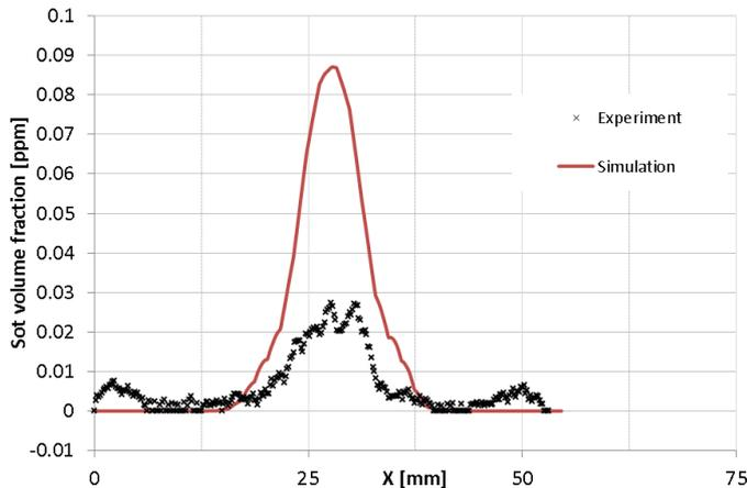
**Figure 12: soot concentration at x=12mm**
