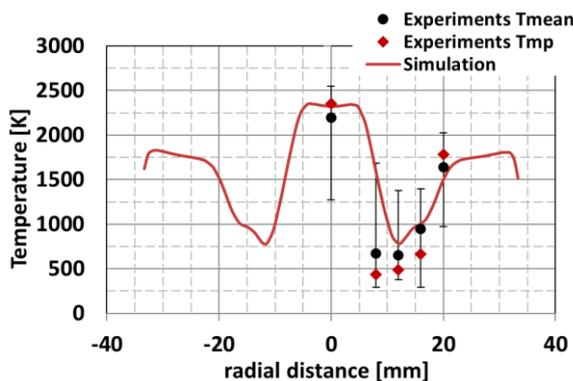
**Figure 9: radial temperature profile at  $x=12\text{mm}$**
