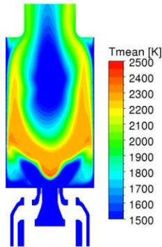
**Figure 8: Time-averaged temperature distribution**
