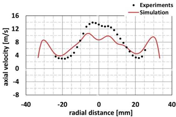
**Figure 7: axial velocity profile at  $x=95\text{mm}$ , i.e. above the secondary air supply**
