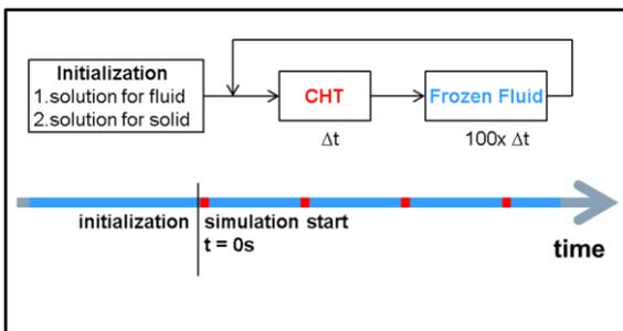
**Figure 1: Scheme of the frozen-fluid process used to speed up the CHT simulation**
