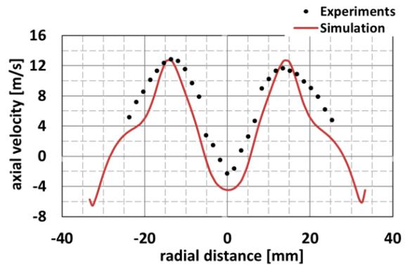
Figure 5: axial velocity profile at  $x=12\text{mm}$
