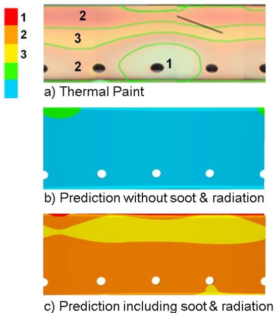
**Figure 15: Combustor wall temperatures for the TECC burner**
