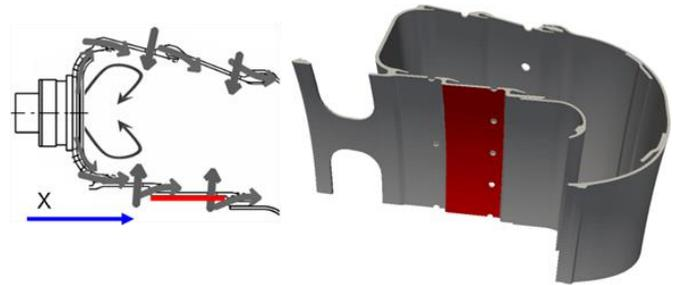
**Figure 14: Scheme and solid domain of the TECC combustor**
