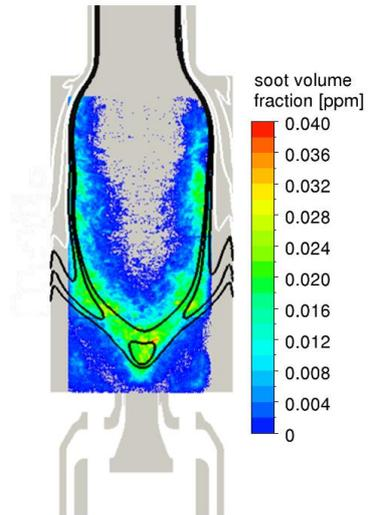
**Figure 11: experimental soot distribution with overlaid isolines**
