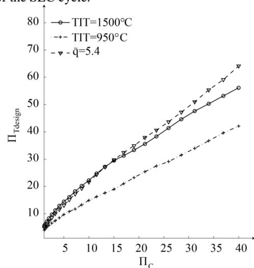
Figure 7. Optimum turbine design expansion ratio in a SEC cycle
