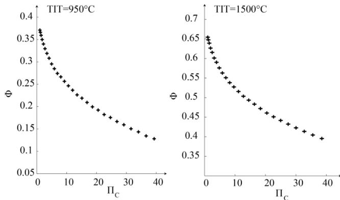
**Figure 8. Equivalence ratio as a function of the compressor pressure ratio a given TIT**
