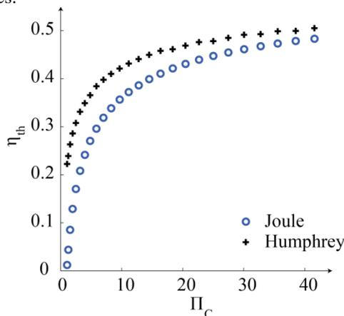
Figure 6. Thermal efficiency of the cycles for dimensionless fuel energy input  $\tilde{q} = 5.4$
