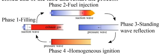
Figure 1 Shockless explosion process
