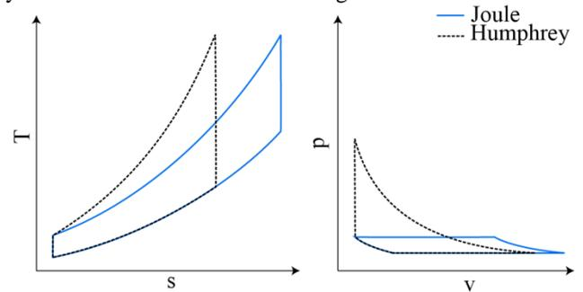
Figure 2. T-s and p-v diagrams of the ideal cycles
