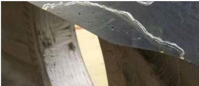
Figure 3 Casting defects at a surface
