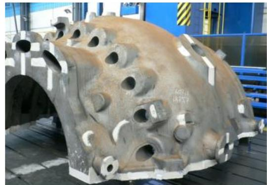
**Figure 1 Casted Turbine housing**
