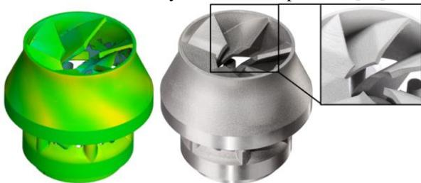
**Figure 7. Axial swirler for the SGT-1000F burner produced by AM (left: nominal-actual comparison)**
