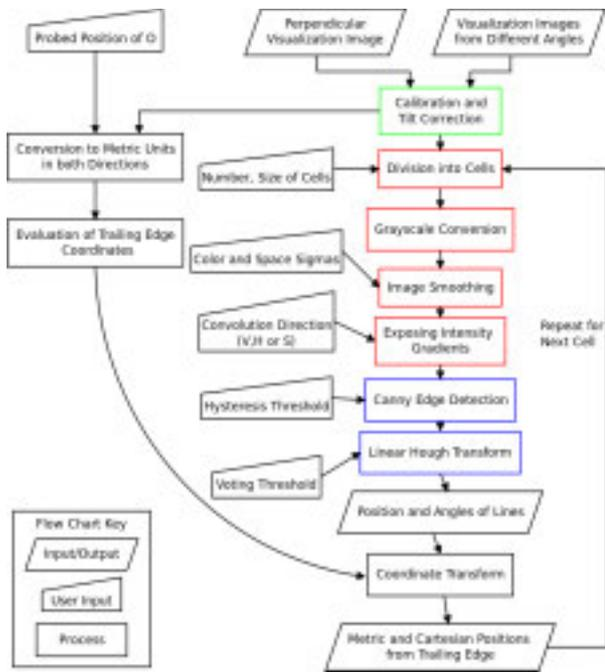
Fig. 2. Flow chart of streakline detection algorithm.
