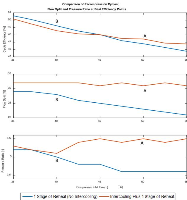
**Figure 3: Flow Split and Pressure Ratio of Maximum Efficiency Point against Compressor Inlet Temperature**
