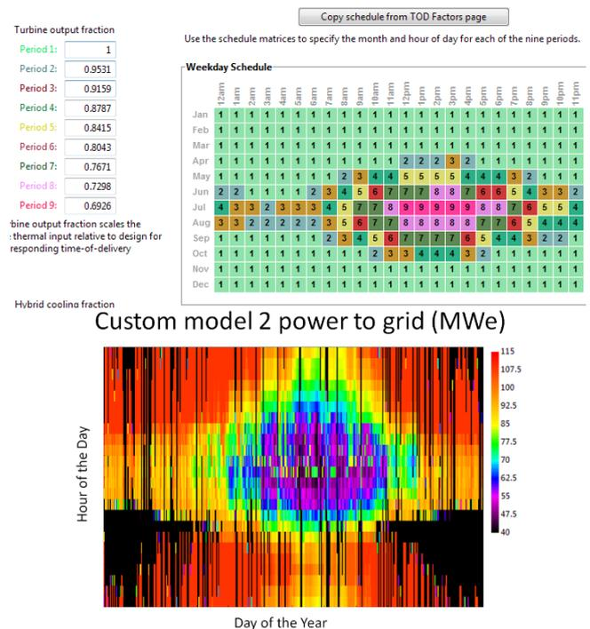
**Figure 6: Schedule Changing Heat Input into the Custom Power Cycle Model and Power Produced**
