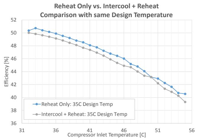
**Figure 4: Comparison of Reheat Only and Intercooling + Reheat at 35°C**
