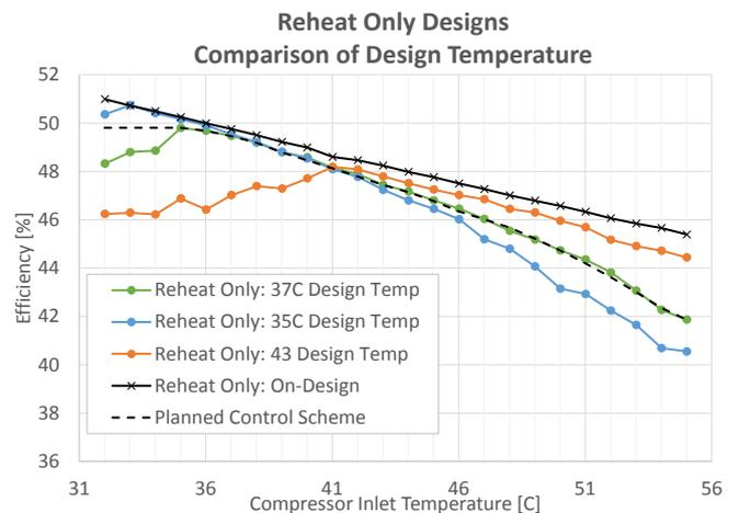
**Figure 5: Comparison of “Reheat Only” Cases at 35°C, 37°C, and 43°C**
