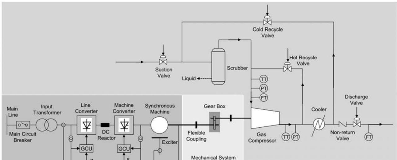
**Figure 3: The electrical and the mechanical subsystems in an electrical compression process**
