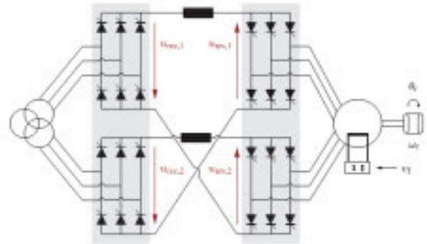
**Figure 1: Variable-speed drive system composed of line-commutated rectifier, inductive DC link, load commutated inverter and synchronous machine.**
