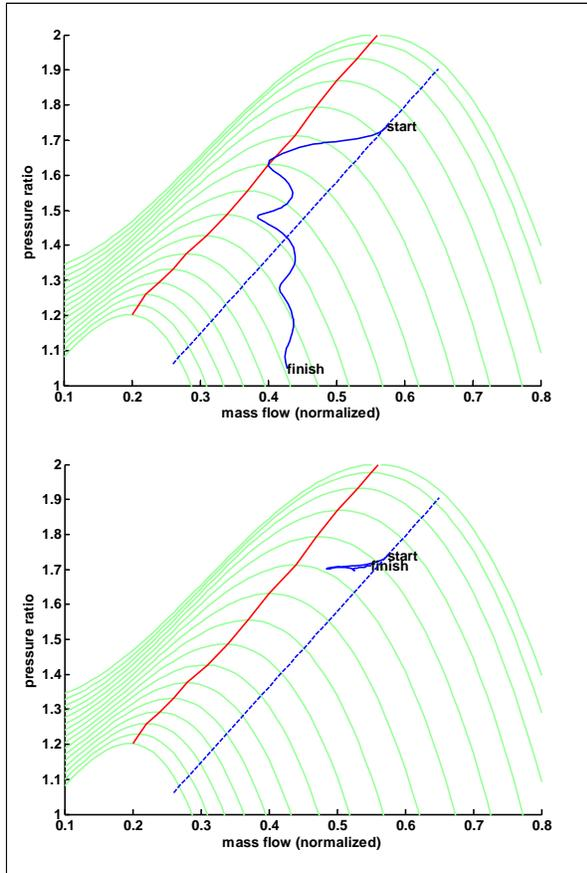
**Figure 4: Simulated trajectories of the compressor operating point during a voltage dip**
