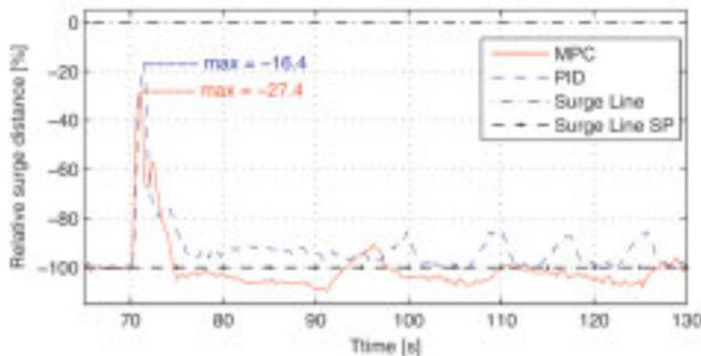
**Figure 4: Simulated trajectories of the compressor operating point during a voltage dip**
