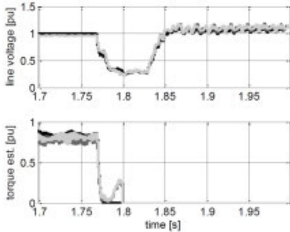
**Figure 2: Estimate of the residual power during voltage dips.**
