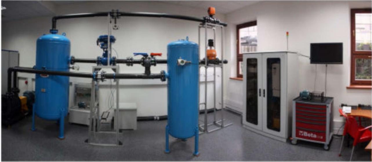
**Figure 5: Electric driven variable speed compressor test rig**
