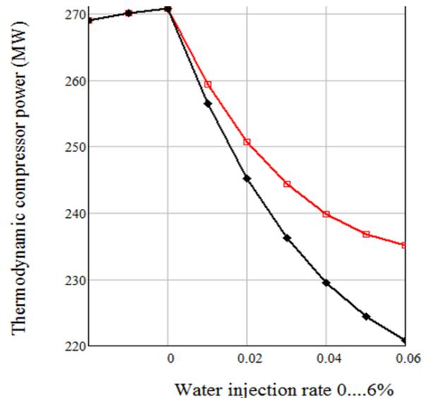
**Figure 4:** Compressor power in the ideal case compared with the calibrated version as implemented in all other figures below. (Black diamond = ideal; red square = empirically calibrated).
