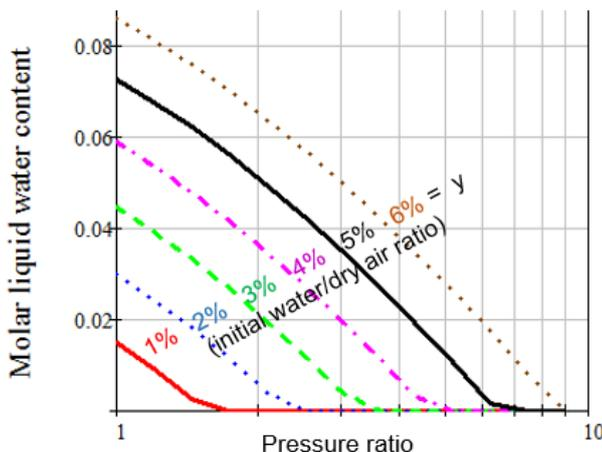
**Figure 1:** Molar liquid water content for wet compression starting at 100% relative humidity and 1.013 bar pressure as a function of the pressure ratio with  $\eta_{pol}=0.912$ .
