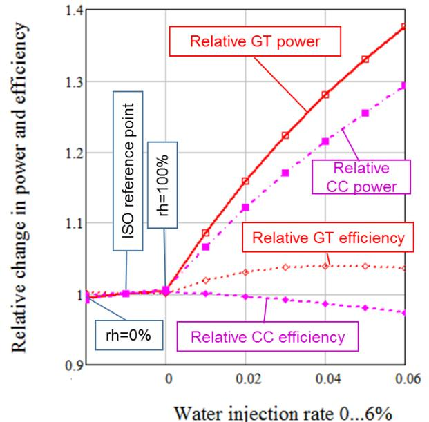
**Figure 2:** Relative performance changes with wet compression of GT and GTCC for equilibrium conditions and maintained polytropic efficiencies (best case).
