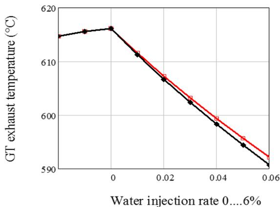
**Figure 11:** GT exhaust temperature as a function of the water injection rate (black diamond = ideal; red square = empirically calibrated)
