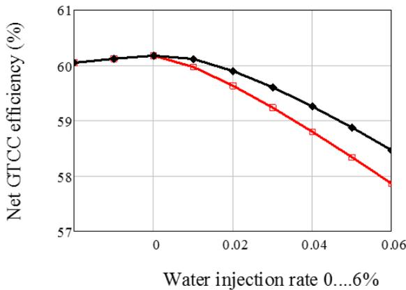
**Figure 6:** Thermal efficiency of a reference GTCC with wet compression (black diamond = ideal; red square = empirically calibrated).
