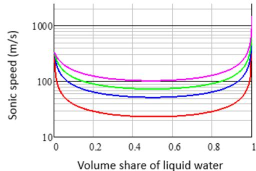
**Figure 13:** Sonic speed of even air-water mixtures at 15°C. Lowest curve for 1bar, above 5, 10 and 20 bar (highest curve).
