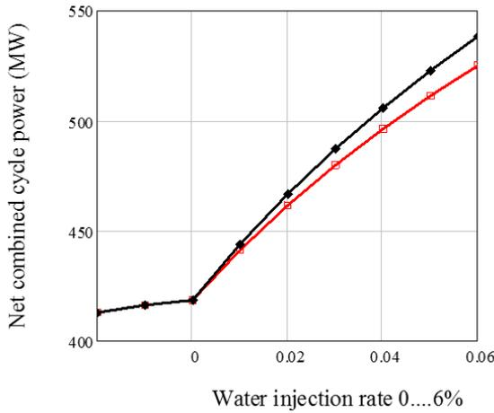
**Figure 5:** Net power output of a reference GTCC with wet compression (black diamond = ideal; red square = empirically calibrated).
