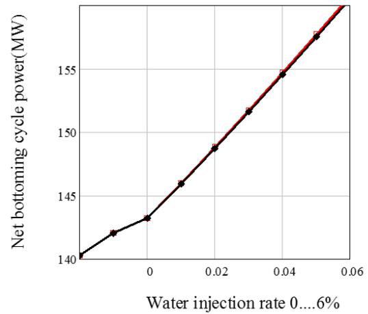
**Figure 8:** Net power of the steam bottoming cycle as a function of the water injection rate (black diamond = ideal; red square = empirically calibrated, both nearly identical).
