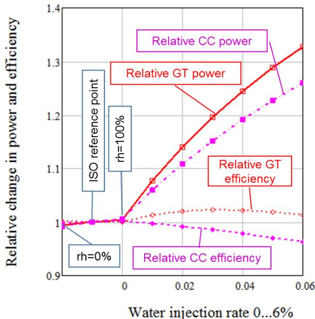
**Figure 3:** Relative performance changes with wet compression of GT and GTCC assuming empiric calibration.
