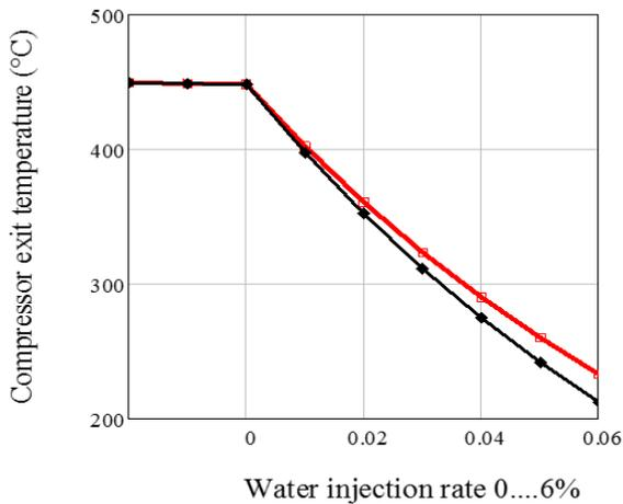
**Figure 10:** Compressor exit temperature as a function of the water injection rate. (Black diamond = ideal; red square = empirically calibrated)
