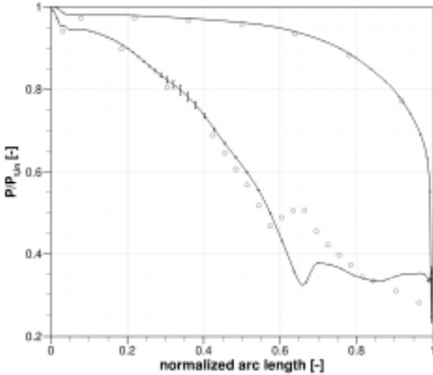
Figure 10: Radial area average and standard deviation of blade pressure in comparison to experimental data
