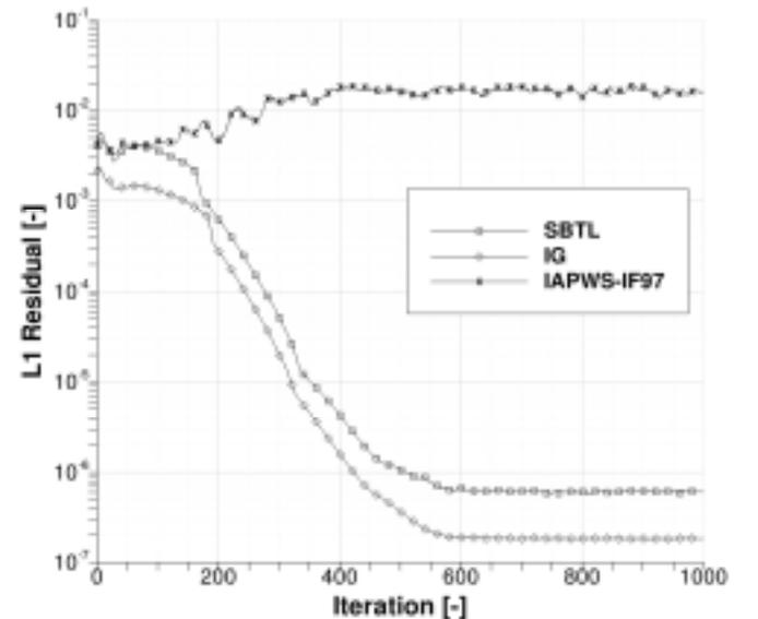
Figure 2: Residuals of the de Laval nozzle calculations
