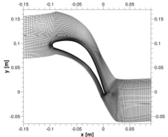
Figure 5: Computational grid for the turbine cascade
