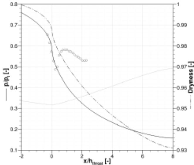
Figure 3: Area averaged axial distributions in the nozzle compared to measured pressure
