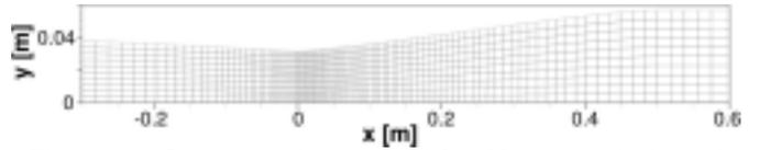
Figure 1: Computational grid for Moore's de Laval nozzle geometry omitting every third cell in each direction
