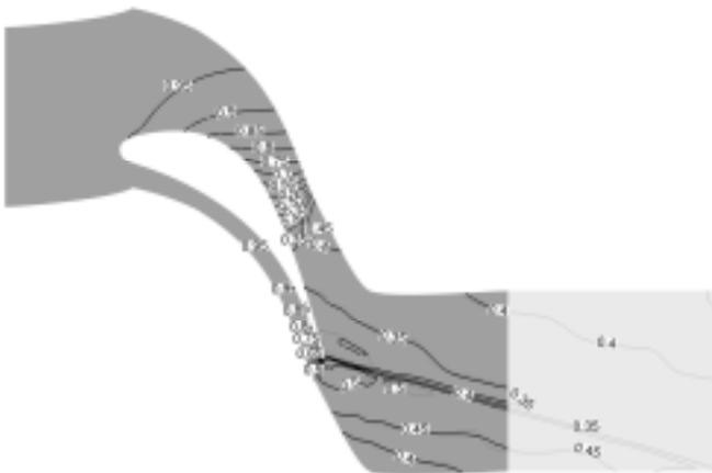
Figure 7: Pressure ratio of small and large domain calculations for the L1 OP
