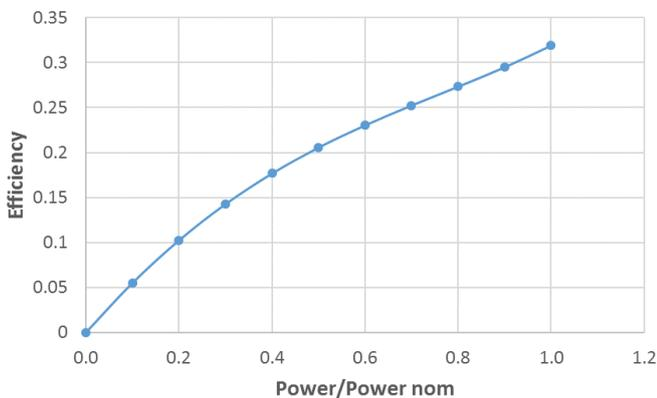
**Figure 2. Gas turbine efficiency as a function of power**
